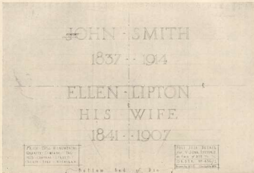
FIG. 41. A TYPICAL FULL SIZE DETAIL FOR LETTERING.
