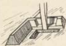
Fig. 5. POSITION OF LETTER- ING BLOCK AND TOOL TO CHIP A STRAIGHT LINE.
