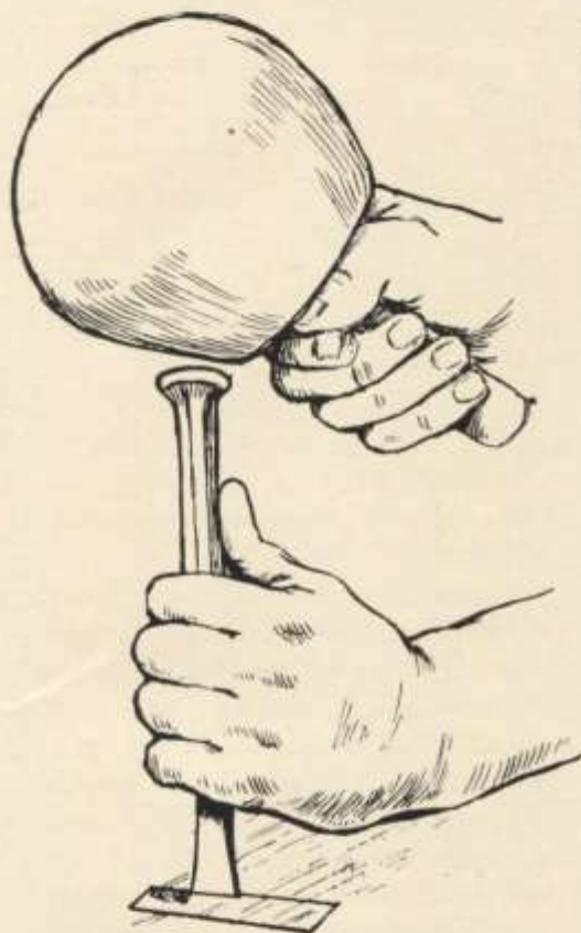
FIG. 32. ROUGHING OUT A STRAIGHT BAR FOR MARBLE SUNKEN LETTER.
