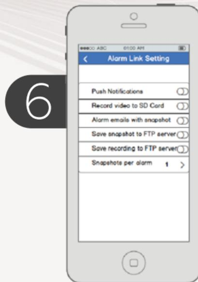
Now that the camera will pick up motion detection, we have to tell it what to do in response. From the Camera Setting page, tap "Alarm Link Setting" to enter the Alarm Link Setting menu.
