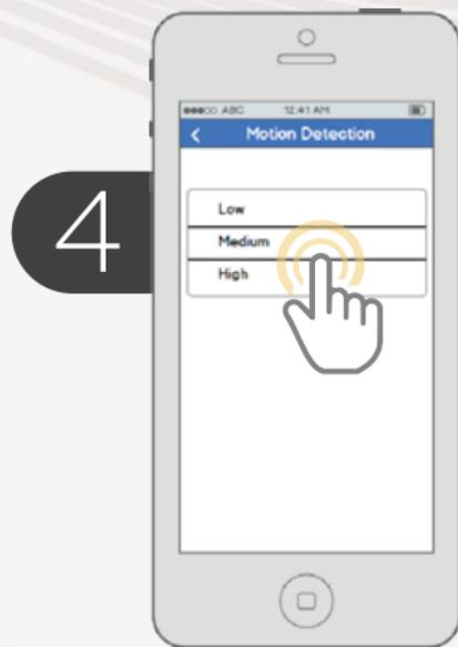
Select a sensitivity for motion detection then tap back to get back to the Alarm Setting menu. The higher the sensitivity, the more easily the camera will pick up movement.
