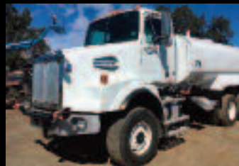
2007 WESTERN STAR 6x6 WATER TRUCK, Cat C13 Acert 410 hp engine, Fuller 8LL transmission, 21,000 lb front 46,000 lb rears w/lockers, Tuftrac suspension, New Randco 4,000 gal water tank with 2 front 1 side 2 rear spray heads, hose reel, plumbed for monitor, 226,140 Miles.....$ 106,500
