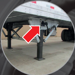
Trailer landing gear can be lubed.
