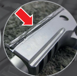
The slide on a gun can be lubed.
