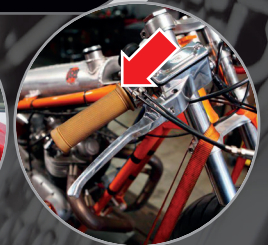
Motorcycle throttle tube can be lubed.
