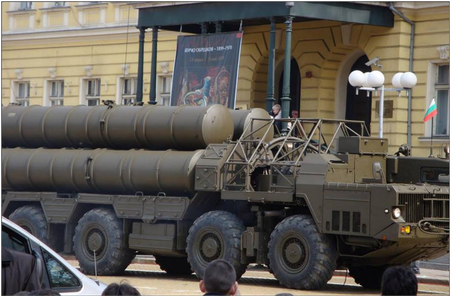
Bulgaria army TEL Transporter Erector Launcher vehicle of S-300 air defense missile system (Picture source Wikimedia).
