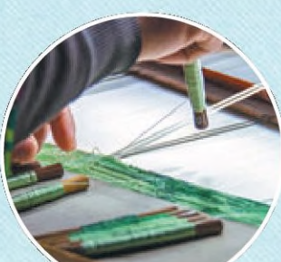
During production, weavers pass a shuttle over and under the alternating warps. PHOTOS PROVIDED TO CHINA DAILY
