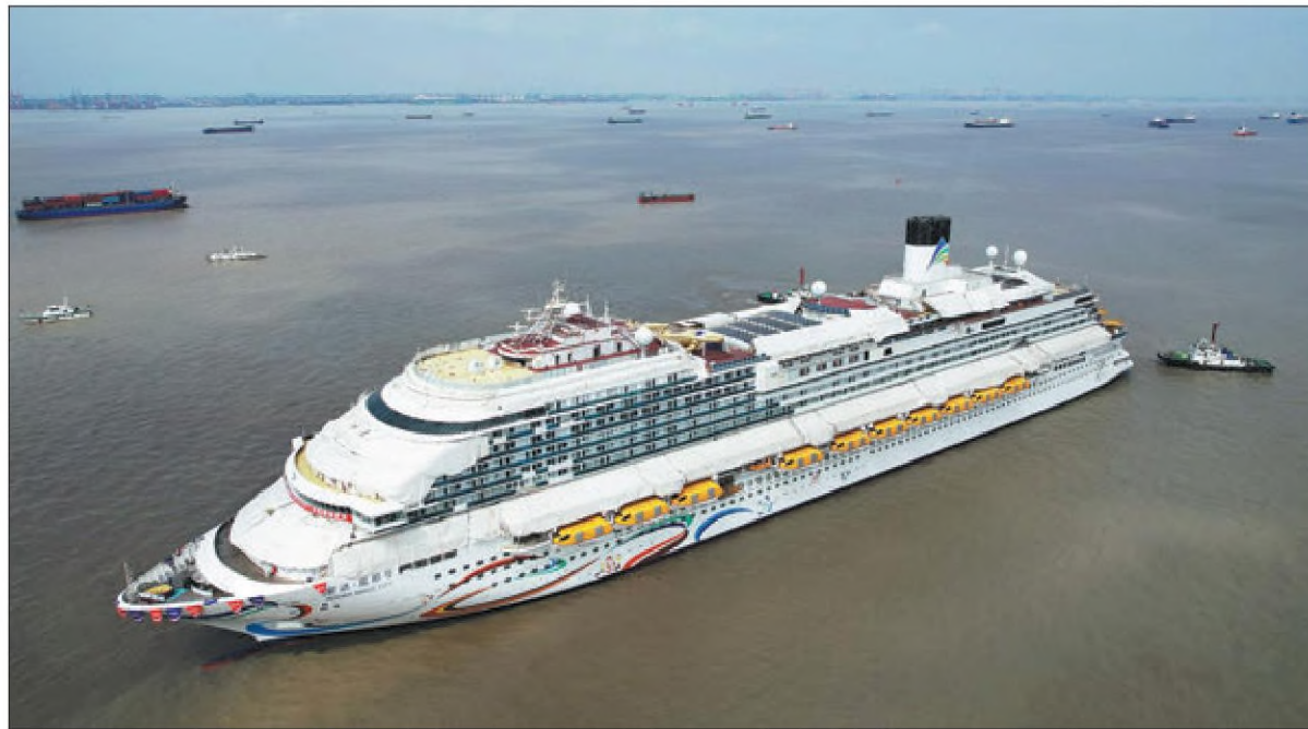
China's first domestically built large cruise ship, Adora Magic City , completes its undocking process in Shanghai on Tuesday. Measuring 323.6 meters in length and 37.2 meters in beam width, the cruise ship can accommodate 5,246 guests. LONG WEI / FOR CHINA DAILY
