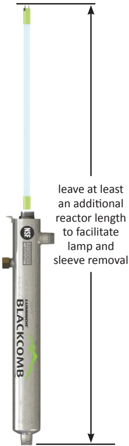
Figure 2. Lamp Removal Spacing
