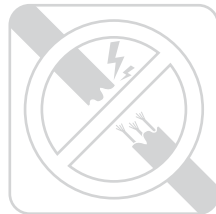
Check for damaged wires
