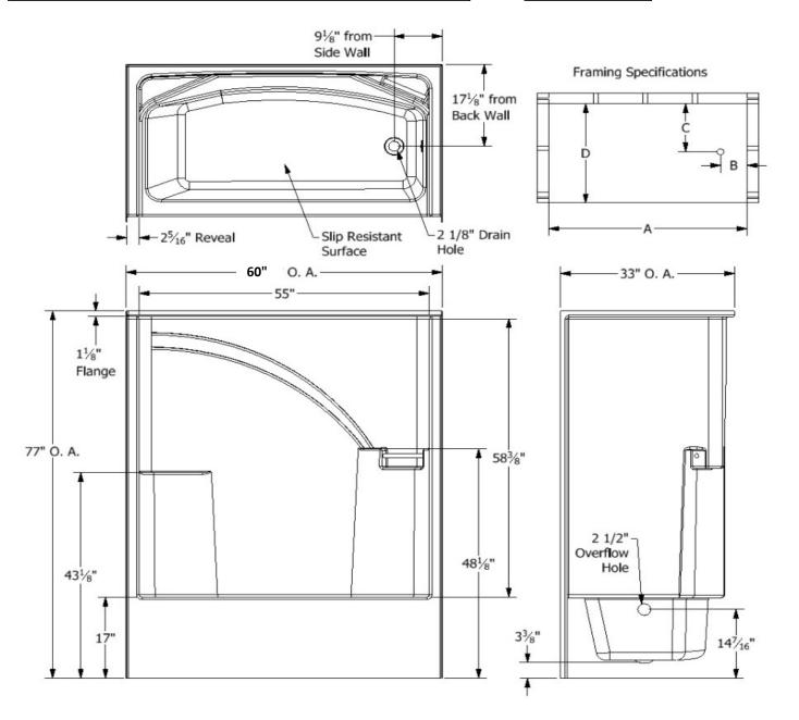
Certified to conform to ANSI Z124.1 and ASTM E- 162 Flame Spread Rating 200 or less and is under a program of factory inspection.
