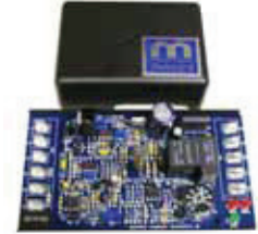
Amplifier, Maxitrol AD1010U, P/N 260864, in Replacement Kit P/N 262321
