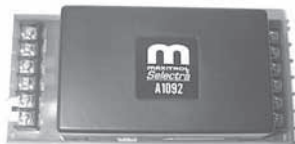
Amplifier, Maxitrol A1010U, P/N 260863, in Replacement Kit P/N 262320
