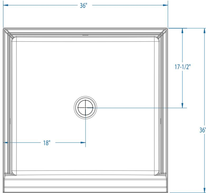
**FEATURES** Dimensional Tolerance  $\pm 3/8"$ . Dimensions needed for site preparation should be measured from the unit. Stream33 assumes no responsibility for preparatory work.
