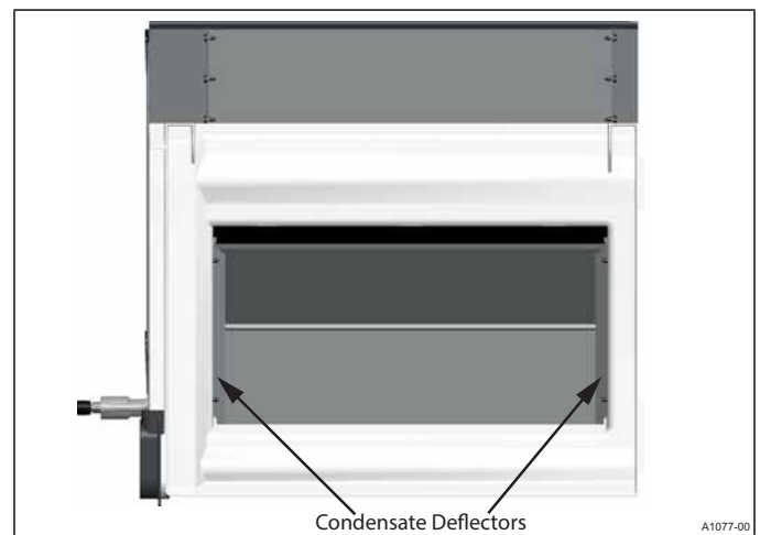
FIGURE 10: 60C Horizontal Right Coil Condensate Final Assembly
