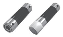
Rugged, precision machined end pieces are held in place by heavy steel collars. Set screws at each end insure that there is no slippage on the shaft flats. Quiet, noise and vibration absorbing, these premium couplings out-perform conventional couplings where misalignment exists or where punishing service is the norm. Available for  $1/2" \times 7/16"$  and  $1/2" \times 5/16"$  shaft sizes, or 7/16" shaft x spline socket.
