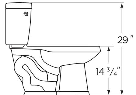
THIS FIXTURE QUALIFIES ACCORDING TO ASME TEST PROCEDURES AS A LOW CONSUMPTION WATER CLOSET WITH AN AVERAGE CONSUMPTION OF 1.6 gpf (6Lpf) OR LESS.
