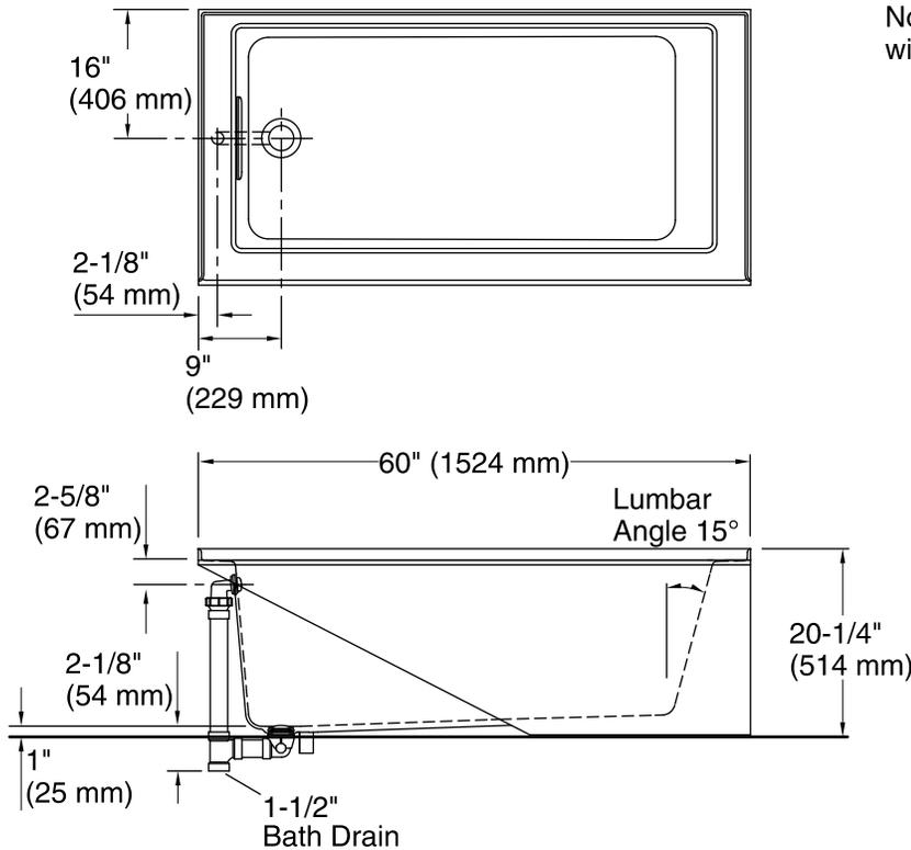
No change in measurements if connected with drain illustrated. (K-7272)
