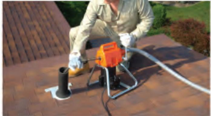
for small drain work, the drum stops turning when you lift the handle to the neutral position.
