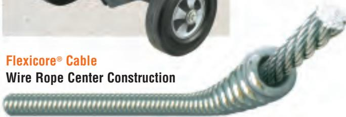
Heavy-gauge wire coiled tightly around 49-strand aircraft-type wire rope and heat treated.
