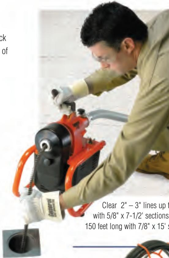
Clear 2" – 3" lines up to 125 feet long with 5/8" x 7-1/2' sections or 4" lines up to 150 feet long with 7/8" x 15' sections.
