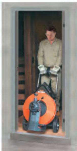
Another important help to you is a see-through inner drum cage so you can tell how much cable is in the drum. For electrical safety, the foot pedal is air actuated, eliminating electrical contact between pedal and motor. Equally important, a Ground Fault Circuit Interrupter senses current leakage and will shut down the machine before an operator suffers an electric shock.
