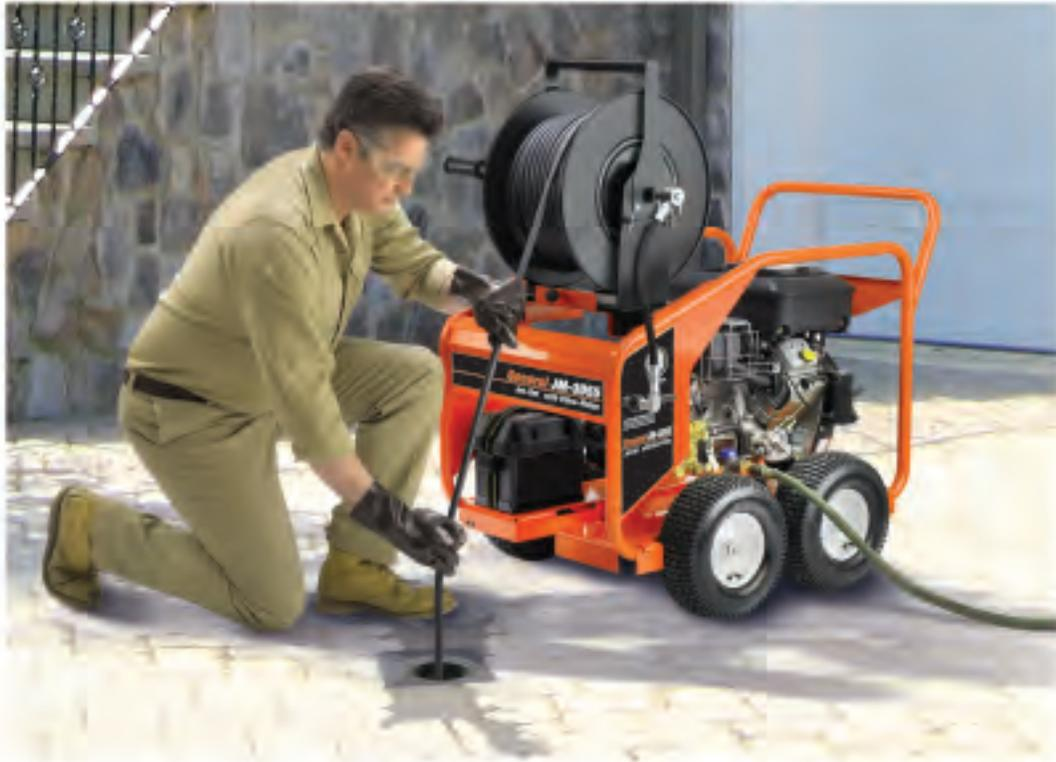
thermal relief valve to protect the pump from heat damage, along with a back flow check valve and inlet filter. Complete with tool box, and spray wand with trigger.
