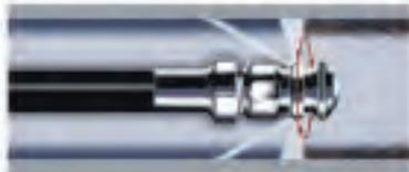
The JN-RB heavy duty hardened stainless steel rotary nozzles have two 90 degree jets to scour the walls of the pipe, and two 35 degree jets to drive the hose down the line. The less expensive JN-RA hardened steel rotary nozzles have two 45 degree jets for combined thrust and cleaning action.
