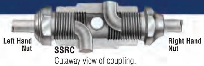
Sectional Rods assemble at right angles and cannot come apart in the line.
