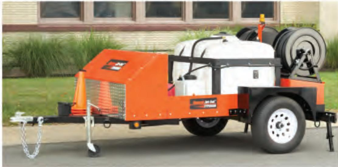
Standard safety features include electric brakes, safety strobe light, three safety cones with holder, rear fold down stabilizer jacks, and retractable guide arm. An anti-freeze system protects the unit from freeze damage. Complete with spray wand and trigger.
