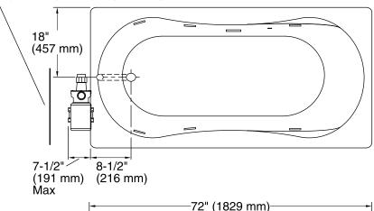
No change in measurements if connected with drain illustrated. (K-11677)
