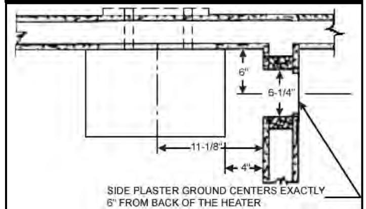
**FIGURE 13 Plaster Ground Installation**
