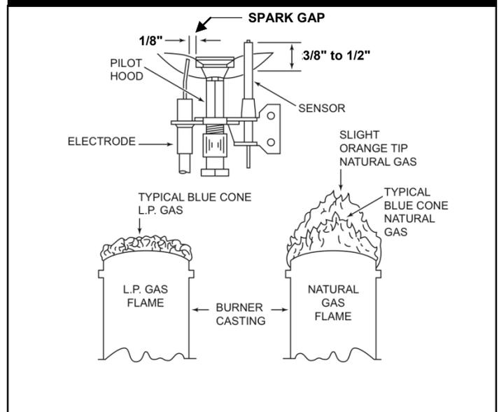
Check the spark gap. It must be carefully adjusted to specifications, as illustrated (Fig. 30), for the ignition device to function properly.
