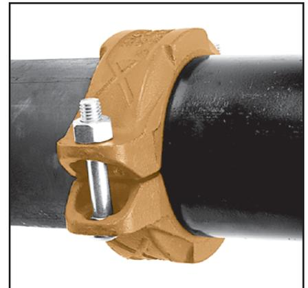
**6 ASSEMBLY IS COMPLETE—** Visually inspect the pipe joint to assure the coupling keys are fully engaged in the pipe grooves. The bolt pads are to have equal gaps on each side of the coupling.
