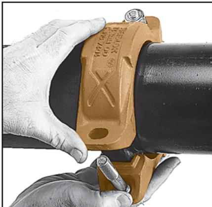
**4 HOUSINGS—** Remove one nut and bolt and loosen the other nut. Place one housing over the gasket, making sure the housing keys fit into the pipe grooves. Swing the other housing over the gasket and into the grooves on both pipes, making sure the tongue and recess of each housing is properly mated. Reinsert the bolt and run-up both nuts finger tight.
