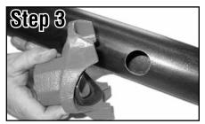
**Gasket installation** Lubricate the exposed surface of the gasket. Align the outlet housing over the pipe hole making sure that the locating collar is in the pipe hole.
