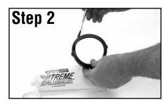
Check and lubricate gasket Check the gasket to be sure it is compatible for the intended service. Apply a thin layer of Gruvlok SPF/Anvil lubricant to the back surface of the gasket. Be careful that foreign particles do not adhere to the lubricated surfaces. Insert the gasket back into the outlet housing making sure the tabs in the gasket line up with the tab recesses in the housing.
