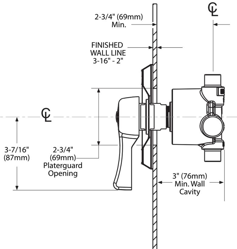
**NOTE:** This valve is not intended to be used as a shut-off valve. To prevent the potential of cross flow, check valves must be integral to the supply valve or installed in both hot and cold water supply lines.
