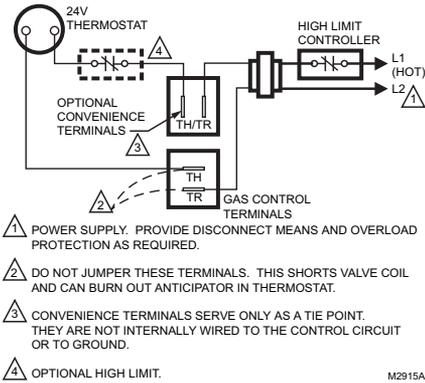
Fig. 8. Wiring Connections.
