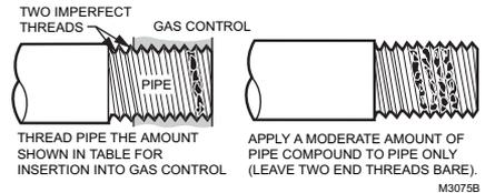
Fig. 3. Use of Moderate Amount of Pipe Compound.
