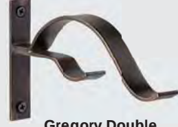
Gregory Double PO138GRDBK ¾" W 3¾" H backplate 6" front return 3" back return Both cradles hold 1½" diameter pole. New Age Bronze
