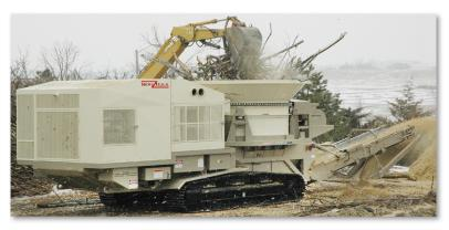
CAT 325L Tracks are Standard Hydrostatic Tracks allow for easier navigation in tight areas.
