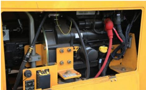
**ENGINE.** The TR6400 features a Deutz 3.6L Tier 4F (Stage IV), 100 hp (75 kW) engine. The engine is mounted on a pivoting frame that swings out 30 degrees for access to fuel filters and hydraulic reservoir for maintenance and service.
