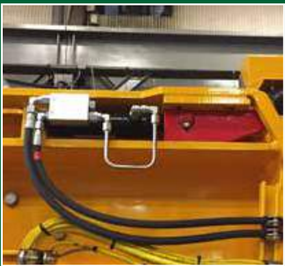
Wedge lock secures upper hog box
