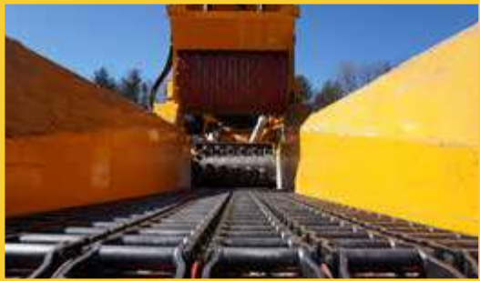
High-torque feed roller. Speed sensors monitor the feed system's speed in real time to maintain a continuous and efficient pace of grinding.
