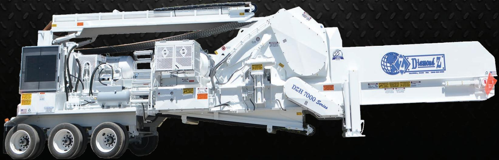
Diamond Z mobile electric grinders house Teco Westinghouse mill drive motors, Teco Westinghouse hydraulic drive motors and a 480 V single soft start control system. These mobile mounting systems create ease of transportation and increases resale value. Diamond Z Electric grinders pack all the punch you expect from a Diamond Z, in an environmentally friendly electric option.
