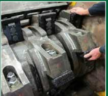
Segmented drum rotor with brute package has twenty striker plates held in place by two 1-1/4" bolts, designed for contaminated demolition debris, railroad ties, and MSW. Striker plates, edged with aggressive carbide, pulverize material and outlast with impressive durability, saving time and money.
