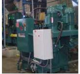
Never get caught empty handed with a blown fuse! Electrical panel employs service friendly molded case and mini circuit breakers for all circuits both main and branch.\*
