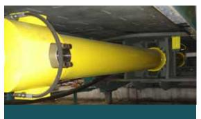
10" main-ram cylinder with up to 353,429 lbs. of platen force delivers up to 40% more force than competitive balers using 10" cylinders.
