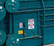
Lower ram chassis inspection door for easy maintenance access.
