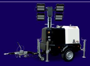
The Generac V20 TowerLight is a mobile lighting tower with four 320 W LEDs on an 8.5 m hydraulic mast that rotates 340°. Powered by a Yanmar diesel engine, it provides up to 143 hours of runtime with low noise, delivering reliable, versatile illumination for construction sites, events, and other large outdoor areas.
