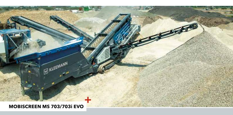
The mobile screening plant MOBISCREEN MS 703 EVO is equipped with a 7 m2 screen box and is used as a double-deck classifying screen. The plant is characterised by favourable transport dimensions and shut setup times. The screen plants are operated by a modern control system. All functions are thus easy to control, operating statuses and machine functions can be viewed at any time.
