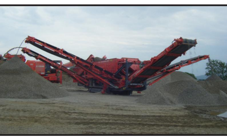
The Terex Finlay 984 is a high performance horizontal 3 deck screener that is easy to set up, versatile and ideal for handling large volumes of material in quarrying, mining and recycling applications.
