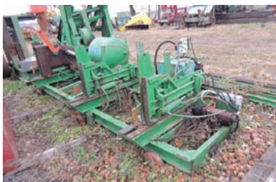
2063 $35,000.00 CIRCLE MILL Cleereman 3 head-block, 36" carriage, Timber Tiger electric set-works, includes track/ drive/ 60" husk/ cab and all controls, in good working condition 260-633-4047
