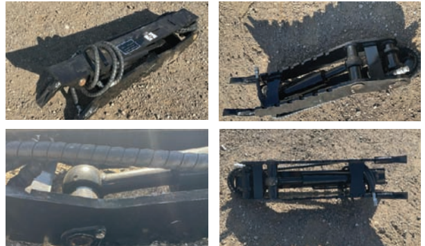
New 2024 Hydraulic Excavator Thumb Fit to CAT 3-5 ton excavator Length 980mm, Maximum clamping force 12KN
