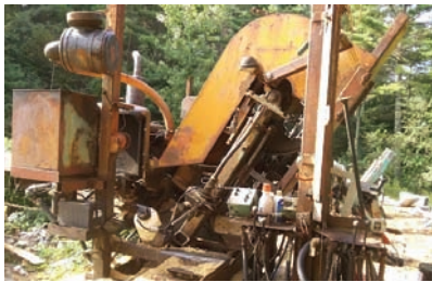
1005S $70,000.00 1984 SANBORN MIN MAX Wide Band Sawmill with Live Deck, Detroit 271 engine with the largest injectors that are made for that engine. It starts and runs well. Includes: hydraulic drive 3 chain live deck that is about 16' long and 12" wide with a stop and loader and arms that go across the bed of the mill. The logs must be rolled across the arms to the 4 head blocks. The frame of the live deck is mounted on 3x3x3 concrete cubes, set of 4 large head blocks with the same design as the original but which are about 12" large capacity than the originals. 40 foot long 3 chain green chain with new hydraulic motor and large gear reduction unit, 3 saw Chase 24" edger with a 271 power unit that starts and runs well. 7 hands here and another 5 being repaired. Many Maintenance and Repairs Done 574-536-1646
