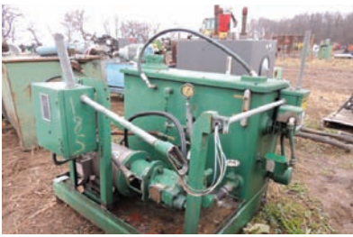
18093 $2,000.00 HYDRAULIC POWER PACK 5 HP. electric motor, has cooling radiator, tank heater, good working condition 260-633-4047
