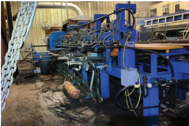
Optimizing Edger Serial #: na. Model: na. # of Blades: 2. # of Moveable Blades: 2. Blade Type: Circle. Cut Capacity: 5" x 36". Drive Type: Electric. Edger Set Up: Stationary. Infeed Measurement: 18' long. Lasers: no. Outfeed Measurement: 19' tailing chain. Features and Notes: (1st of an entirety) 2 saw optimizing etcher with Inavec scanning system, Inavec feed system,.
