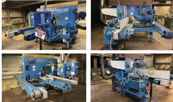
Brewer Band Resaw Serial #: 031496. Model: 1B8X12-2000. # of Heads: Single. Blade Size: 1 1/4". Blade Tension: Air. Cut Capacity: 6" x 12". Drive Type: Electric. Guide Type: Roller. Overall Dimensions: 9' x 14'. Return: yes. Wheel Size: 1 1/2" x 36". Features and Notes: 8" x 13'6", feed and return w/6" belt, hydraulic drive, 5 hp electric hydraulic pack, live press down wheel.
