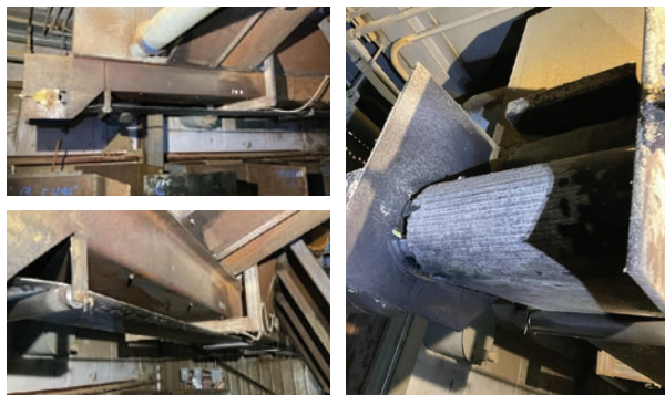
Belt conveyor Length: 94'. Belt Width: 18". Drive Type: Electric. Overall Width: 25". Features and Notes: 10" sides, no support legs.
