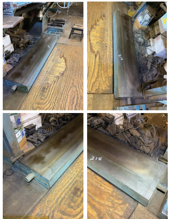
Hammering Anvil Bottom anvil, 14" x 5' x 4 3/4"
