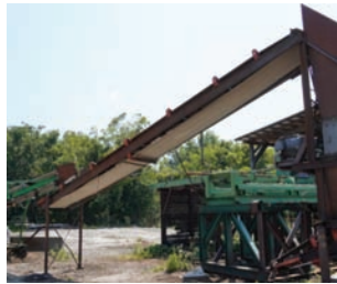
9219 CONCAVE BELT CONVEYOR $7,000.00 36" wide x 30' long, electric gear box drive, good working condition 260-633-4047
