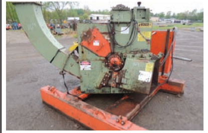
7148 CHIPPER $32,500.00 48" 6 knife chip-pac, includes 5' x5' shaker screen, electric drive, includes soft start, numerous spare knives and parts, good working condition 260-633-4047
