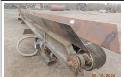
9167 BELT CONVEYOR $500.00 4" wide x 15' long, approx 4" tall sides, electric drive, good working condition 260-633-4047
