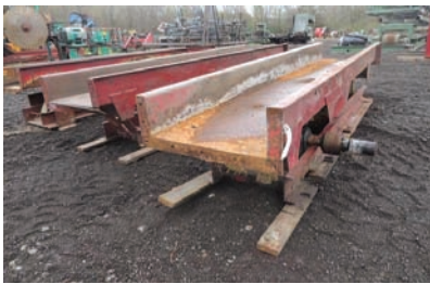
9236 VIBRATING CONVEYOR $10,500.00 30' L, hyd drive, 24" pan, 8" sides, 19" from floor to bottom of pan, good condition 260-633-4047
