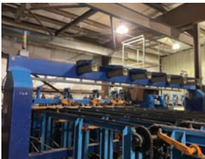
Optimizing Edger Serial #: na. Model: na. # of Blades: 2. # of Moveable Blades: 2. Blade Type: Circle. Cut Capacity: 5" x 36". Drive Type: Electric. Edger Set Up: Stationary. Infeed Measurement: 18' long. Lasers: no. Outfeed Measurement: 19' tailing chain. Features and Notes: (1st of an entirety) 2 saw optimizing etcher with Inavec scanning system, Inavec feed system,.
