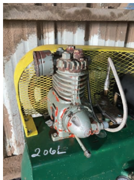
Devilbiss Air Compressor 1.5 hp, 3 phase motor, on tank.
