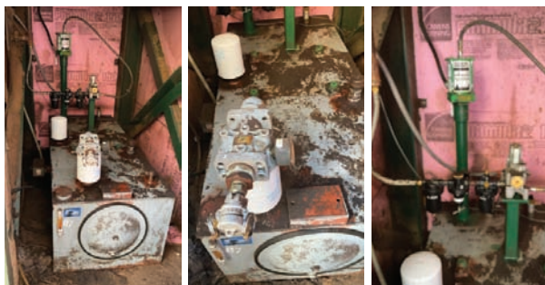
Nicholson Auto Oiler (Part of an entirety) Air powered oiler for debarker, 5' x 27' x 21' tank.
