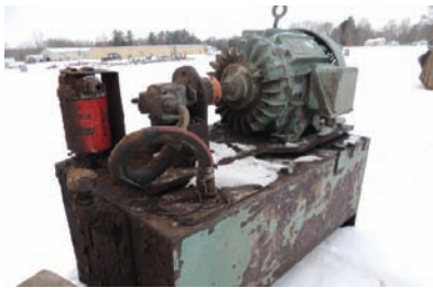
18215 HYD UNIT $1,700.00 15 hp electric motor, vane type pump, approx 80 gal capacity reservoir, good working condition 260-633-4047
