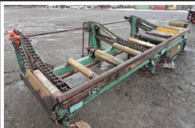
9125 TRANSFER DECK $2,750.00 roll case with transfer, 24" wide x 12' long roll case, 3 strand pop-up transfer deck 10' 6" wide x 5' long, electric drive, working condition 260-633-4047
