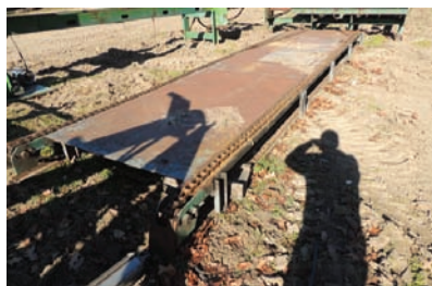
9095 TRANSFER DECK $5,000.00 2 strand transfer deck, 5' wide x 23' long, 81XH chain, BRAND NEW DRIVE SHAFT/ SPROCKETS, very good condition 260-633-4047
