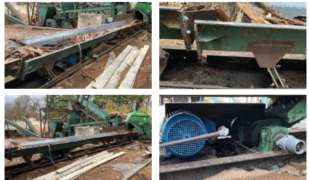
Vibrating Conveyor Drive Type: Electric. Overall Dimensions: 36" x 25'. Pan Width: 24".
