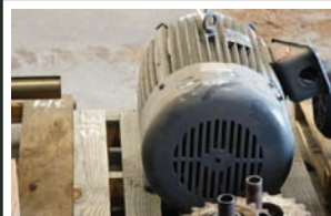
Electric Motor Rebuilt 30 hp electric motor
