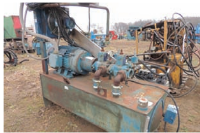
18186 HYDRAULIC PACK $5,000.00 30 HP electric motor w/double pump direct mounter, approx. 100 gal tank, lots of electric control valves, oil cooler, electric control box 260-633-4047
