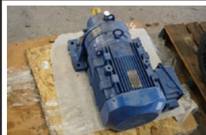
New Electric Motor 10 hp electric motor
