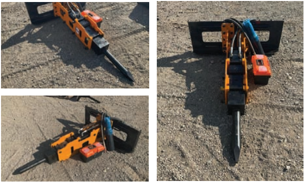
New 2024 Skid Steer Breaker Total length (mm) 1830, Driving oil pressure (kg/cm²) 95-130 Drive oil volume (L/min) 30-45, Strike rate (bmp) 450-750 Drill rod diameter (mm) 68
