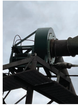
Dust Blower Serial #: na. Model: na. Drive Type: Electric. Includes Pipe: yes. Inlet Size: 12". Outlet Size: 12". Features and Notes: Includes pipe to blower and to cyclone, 12" x 50' steel pipe, includes steel frame blower sits on.
