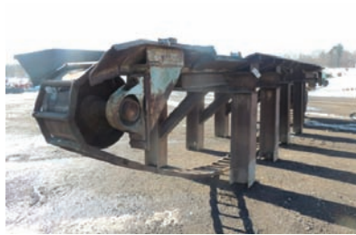
9090 $14,300.00 LOG TROUGH 40' long, 110 ladder-back chain, 14" wide, s- style drive, no power, good working condition 260-633-4047
