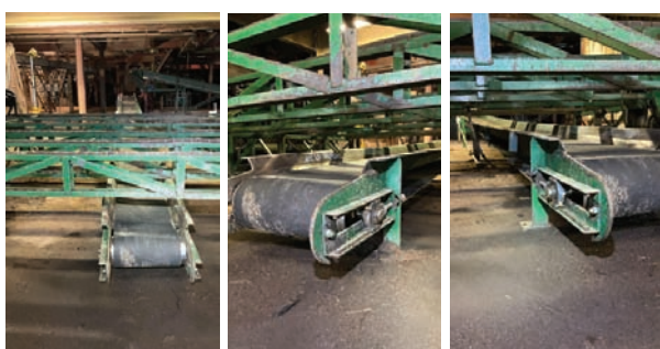
Belt Conveyor Length: 41'. Belt Width: 18". Drive Type: Electric. Overall Height: 48". Overall Width: 26". Features and Notes: 4" sides, on incline.
