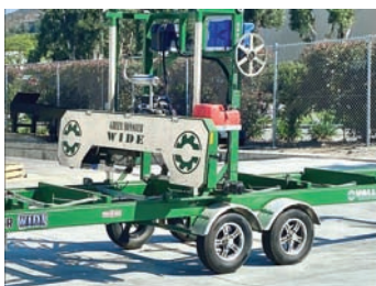
1165A $16,000.00 M & M VALLEE GREEN MONSTER WIDE PORTABLE SAWMILL ENGINE -22 HP Honda GX690 - 50.1 cutting hrs SAW HEAD -Maximum log diameter / board width of 42" - 1 1/4" last board cut capability-Blade of 203x1 1/2 APEX RF (10 blades included)-Electric Saw Head positioning & auto-lock electric winch of 4000 lbs mounted on a drum shaft w/double cables of aeronautical quality- Hydraulic blade tensioner w/pressure indicator-High grade triple bearing blade-guide, Zinc design & adapted for heavy usage, w/20" wheels- Large 7 gallons (26 liters) removable lubrication tank BASE -Up to 21' maximum board length, onto a 24' bed - Extra solid steel tubing frame 2X6 3/16, welded w/crosspieces, no joints - 2 log clamp, simple one hand cam-lock design-4 adjustable jacks & 5 stabilizing legs for maximum stability TOWING EQUIPMENT- 3000 lb suspension axles, alloy wheels, high quality tires & wheel fenders - Drawbar w/2 inches trailer tongue, & 3500 lb security chain 760-798-5410
