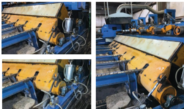
Board Tipple (Part of an entirety) 18' capacity air operated.
