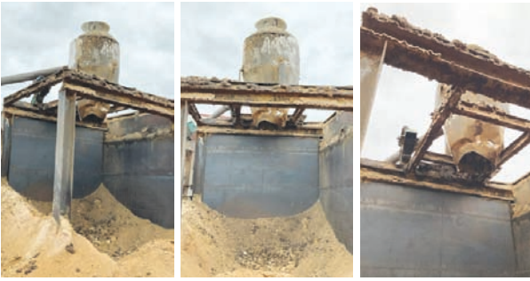
Dust Cyclone and Steel Frame 5' stainless steel cyclone, 12' x 12' steel sides for dustbin, 2 sides are solid steel.
