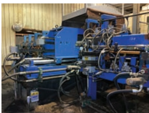
Optimizing Edger Serial #: na. Model: na. # of Blades: 2. # of Moveable Blades: 2. Blade Type: Circle. Cut Capacity: 5" x 36". Drive Type: Electric. Edger Set Up: Stationary. Infeed Measurement: 18' long. Lasers: no. Outfeed Measurement: 19' tailing chain. Features and Notes: (1st of an entirety) 2 saw optimizing etcher with Inavec scanning system, Inavec feed system,.
