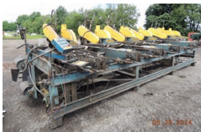
17106 $42,500.00 MULTI HEAD TRIM SAW Newman KM-16 6 head trim saw, hyd drive, includes 2 belt conveyors, all controls, ready for production 260-633-4047
