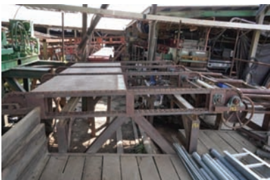
9227 TRANSFER DECK $3,750.00 4 strand transfer deck, 10' 6" x 10' long, H-78 rooftop chain, electric gearbox drive, has board stops, good condition 260-633-4047
