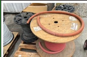
Radiator and Rubber Line 1" DuraFlex 250 PSI, 6.3 mm 1/4" 350 PSI hose, 500 W CSA 600 V coated wire
