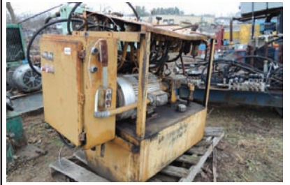
18210 HYD UNIT $2,000.00 used on Fulghum rosser-head debarker, 15 hp electric drive, 2 stage vane type pump, approx 45 gal tank, working condition 260-633-4047
