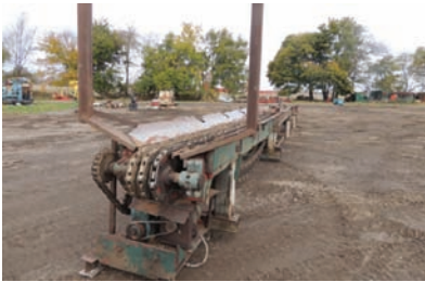
9087 $20,000.00 LOG TROUGH 55' long, 12" pan width, electric drive, good working condition 260-633-4047
