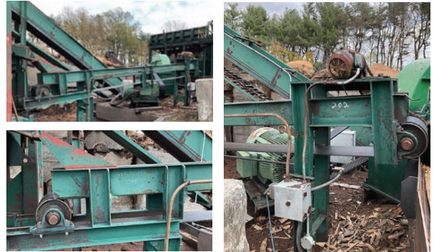
Belt Conveyor (Part of an entirety) Length: 20'. Belt Width: 12". Drive Type: Electric. Overall Height: 80". Overall Width: 17".
