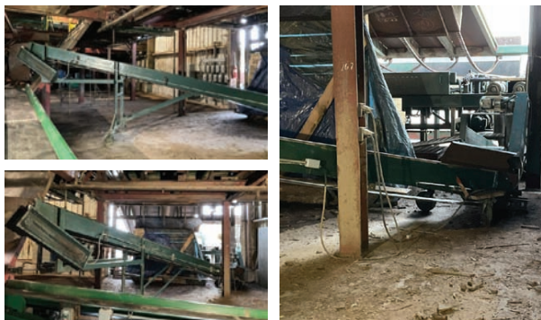
Belt conveyor Length: 30'. Belt Width: 16". Drive Type: Electric. Overall Height: 8". Overall Width: 22". Features and Notes: 10" sides, on wheels for portability.
