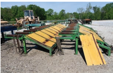
9205 $4,000.00 ROLL CASE Roll case/ transfer deck, rolls are 30" wide x 38' long total length, transfer is 52" wide and 38' long, lighter duty and in good working condition 260-633-4047
