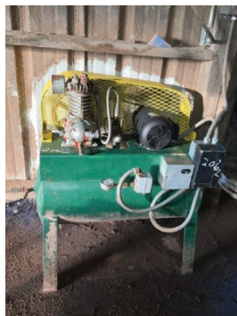
Devilbiss Air Compressor 1.5 hp, 3 phase motor, on tank.
