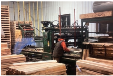
14001S $47,500.00 1987 VIKING CHAMPION 304 PALLET NAILER "Viking Pallet Nailer model Champion 304, Four (4) head with stacker and rolls. Comes with hydraulic pump. Will need air compressor. Good working condition. Call 800-459-2148 for more info." 574-536-1646
