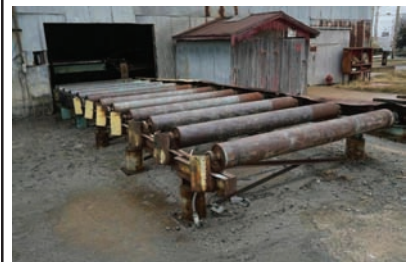
9229 ROLL CASE $15,000.00 90" wide x 28' long, electric drive, heavy duty and in good condition 260-633-4047
