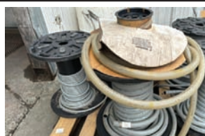
Hose Hydraulic line 16 bar/250 PSI, rubber line 801-16wp 1.2 mp (175 PSI), rubber line 801-12 wp 1.7 mp (250 PSI), rubber line 801-3-GRA-WPA 2.1 mp(300 PSI)
