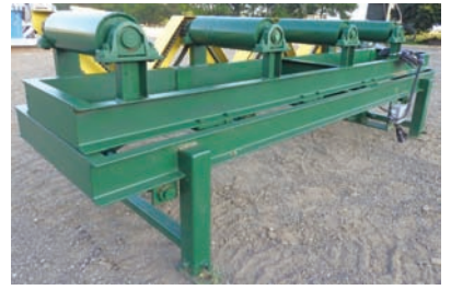
9217 ROLL CASE $4,500.00 pop-up rollers, perfect for putting in a transfer deck, 16" wide x 7' long, foot pedal control, hyd drive, BRAND NEW! 260-633-4047
