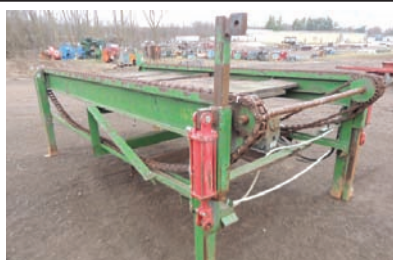
9164 TRANSFER DECK $3,250.00 2 strand transfer deck, 5' wide x 12' long, H-78 chain, electric drive, board/ cant stops hyd operated, good working condition 260-633-4047
