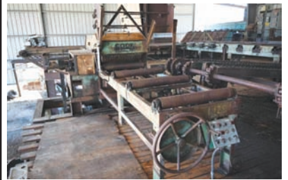
5114 COOK EDGER $10,750.00 Model:36EZTD, SN: 42, 5" x 21' tailing belt outfeed, 38" x 9' infeed rolls, 6" x 36" infeed cap, control panel, manual blade set, (2) 20" blades both are adjustable, electric drive, good heavy duty older unit 260-633-4047
