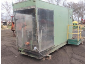
20300 OPERATOR CAB $5,500.00 Operator/ sawyer cab, 4'6" wide x 13' long x 7' tall, includes air-ride seat, good condition 260-633-4047
