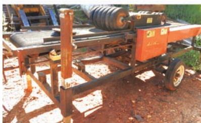
5601 $4,500.00 TIMBERKING EDGER 2x21 bd. Edger. 2 blade 1 movable, with another spacer. Infeed & outfeed belt with pressdown roller. 20 HP gas motor. In Good working condition. Write Riverside Hardwoods 663 McAtee Rd. Cadiz, KY. 42211 270-498-8454
