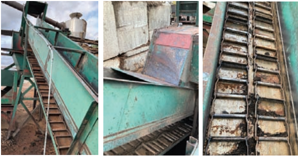
Chip Conveyor (Part of an entirety) 29" x 35', 22" sides, dual ladder back chain, electric drive.
