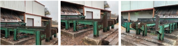
4 Strand Transfer Deck # of Strands: 4. Drive Type: Electric. Overall Dimensions: 11' x 21'. Features and Notes: Steel frame on end.
