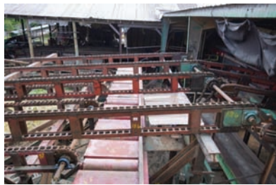
9225 TRANSFER DECK $4,500.00 4 strand transfer deck, 10' wide x 14' long, H-78 chain, gear box drive, includes board tippie at end of deck, good working condition 260-633-4047
