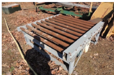
9151 ROLL CASE $650.00 light duty roll case 52" wide x 60" long, electric drive, 2 1/2" dia rolls, working condition 260-633-4047
