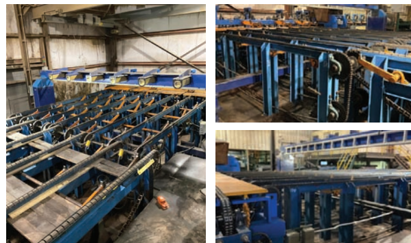
Infeed Deck (Part of an entirety) Board stops, no drive.
