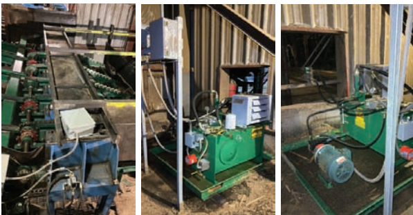
Rollcase with Side Transfer Drive Type: Hydraulic. Overall Dimensions: 21' x 8'6". Roller Size: 9" x 24". Features and Notes: 5 strand side transfer with cleats welded to chain, roll off, dead rolls, includes hydraulic pack.
