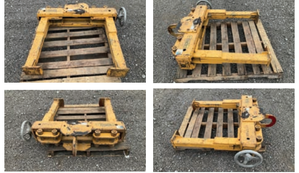
5 Ton Lifting Clamp Model: 83HWS-5-24, Rated capacity: 10,000 lbs. Contact Daniel Miller with any questions 440-321-5965
