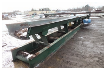
9119 VIBRATING CONVEYOR $13,750.00 Jeffrey vibrating conveyor, 18" wide pan x 36' long, 6" tall sides, electric drive, good working condition 260-633-4047
