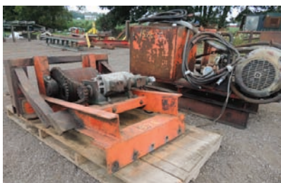
18200 CARRIAGE DRIVE $4,000.00 40 hp electric drive, approx 125 gal reservoir, includes cable drum and motors, good condition 260-633-4047
