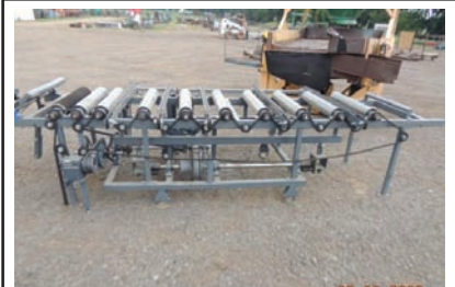
9080 $5,000.00 ROLL CASE/TRANSFER roll case with transfer, 26" wide x 11' long, 5 strand pop-up transfer, all mechanical and line shaft ready, like new condition 260-633-4047
