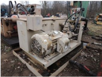
18153 $4,000.00 HYD. UNIT GS hyd. unit, 25 HP. electric drive, 2 pump sections, one is a pressure compensated, very good condition 260-633-4047
