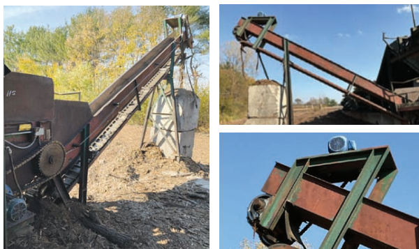
Chain Bark Conveyor 20' x 26', 17" pan, 11" ladderback chain, electric drive, elevated.
