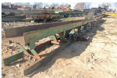
9078 $15,000.00 VIBRATING CONVEYOR Morbark 17" wide pan x 37' long, 6" tall sides, has fines section, chipper infeed spout, good condition 260-633-4047
