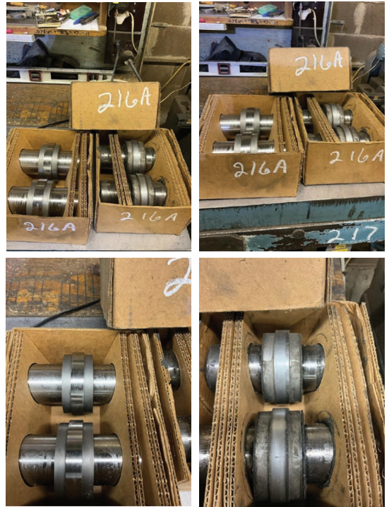
Armstrong Rollers 2 new and 2 used rollers for Armstrong stretcher roller
