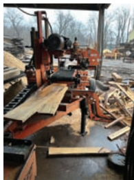
1010S $45,000.00 2001 WOOD-MIZER LT40 SUPER HYDRAULIC SAWMILL with re-saw attachment with setworks, Replaced the hydraulic motor for the re-saw and replaced the guides. 25HP Electric Motor. Road ready. Can be switched to portable power - costs around $4000-$5000 from Wood-Mizer. Call 800-459-2148 for more info." 574-536-1646
