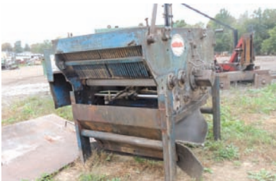
5116 BOARD EDGER $14,250.00 Cornell 4" thick x 27" wide capacity, 1 stationary-1 movable blade, includes infeed, this edger is in good working condition 260-633-4047
