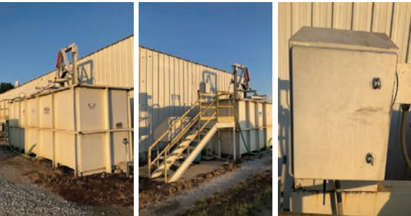
Lumber Dip Tank 7' x 21', stainless steel, remote controlled lift, hydraulic pack
