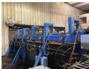
Optimizing Edger Serial #: na. Model: na. # of Blades: 2. # of Moveable Blades: 2. Blade Type: Circle. Cut Capacity: 5" x 36". Drive Type: Electric. Edger Set Up: Stationary. Infeed Measurement: 18' long. Lasers: no. Outfeed Measurement: 19' tailing chain. Features and Notes: (1st of an entirety) 2 saw optimizing etcher with Inavec scanning system, Inavec feed system,.
