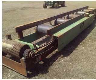
9187 $3,500.00 ROLL CASE 24" wide x 19' long, hydraulic drive, very good condition 260-633-4047
