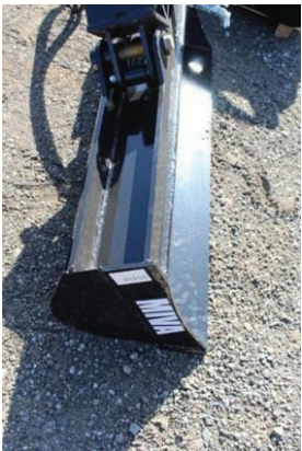
New 2024 MIVA 40" Titling Bucket Fits a 1-3 ton excavator, pin diameter 1"
