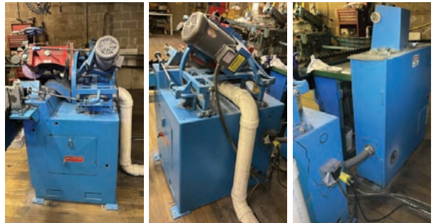
Armstrong Bandsaw Sharpener (1st of an entirety) Model #4 B. S. S., SN: 20557, Vari Sharp, right hand, 480 V, 3 phase, updated vertical sliding head, 3 sets cams
