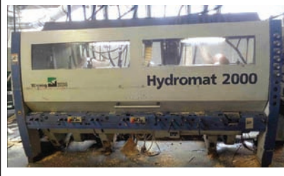
20169A $50,000.00 2008 WEINIG HYDROMAT H-2000 5-HEAD HI-SPEED MOLDING Hyd, hi-speed horizontal ripping, planing or moulding w/feed speed up to 330 FPM, 5 heads installed (originally 7-head), Standard 9" width. Auto Waxlit bed oiler. Includes feed rolls, tooling, spare parts, & hydraulics & dust collection manifold, Well- maintained, still used daily ! Come check it out prior to 8/26. More equipment coming up for grabs soon. 570-758-2597
