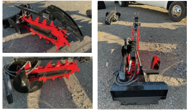
New 2024 GIYI GY-X380 Mini Trencher Trenching width: 150 mm, Trenching depth: 950 mm, Number of Teeth: 16, Maximum flow: 57L/MIN, Working pressure: 10-22 MPA
