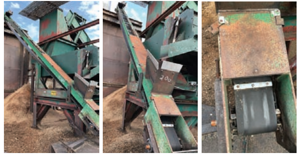
Fines Belt Conveyor (Part of an entirety) Length: 25'. Belt Width: 8". Drive Type: Electric. Overall Width: 11". Features and Notes: No support frame.
