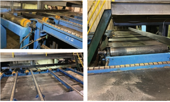
Live Rollcase (Part of an entirety) Drive Type: Hydraulic. Overall Dimensions: 64" x 22'. Roller Size: 9" x 50". Shaft Size: 1 15/16". Features and Notes: Each roll is individual drive.
