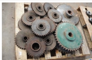
Chain Sprockets Assorted chain sprockets, some with bearings, arbor size 1 7/8"-2"
