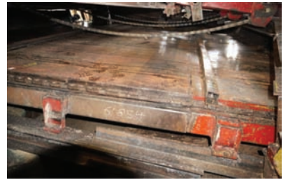
9220 SLAB DRAG DECK $8,500.00 slab drag, 15' x 15', electric gearbox drive, 81X chain with steel cleats bolted on, good working condition 260-633-4047
