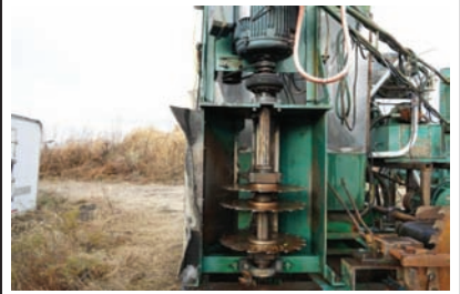
5107 VERTICAL EDGER $13,500.00 Cedar Creek, 3 blade, 6" capacity, 30 hp electric drive, good condition 260-633-4047
