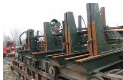
2078 $47,500.00 CLEEREMAN 4 HB MILL Cleereman 4 head block , Model 40, air over air setworks, includes cab/track-frame/ carriage drive and all controls, in good working condition 260-633-4047
