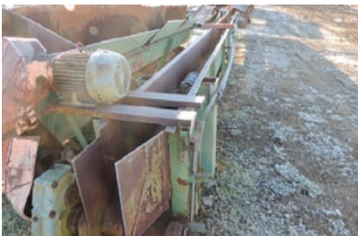
9142 WASTE CONVEYOR $8,500.00 10"x60' waste conveyor H78 chain with paddles, electric drive ,includes new chain 260-633-4047
