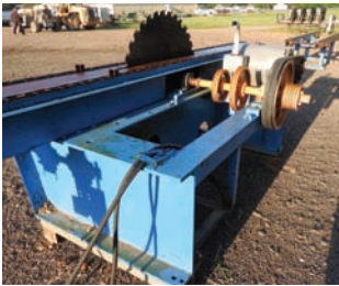
2094 $5,000.00 SPLITTER SAW designed to split cants, boards, etc., 50hp electric drive, 81x chain, 40" dia inserted tooth blade, hyd drive on feed, good working condition 260-633-4047
