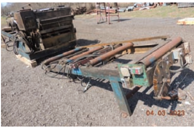
5111 CORNELL EDGER $17,250.00 6" x 42" capacity, MN: HE42, SN: 703-10-81, single arbor, (4) 19" saws, 2 movable blades, 8' infeed, 8' powered outfeed, electric drive, comes w/ spare spacers, saws and laser lights 260-633-4047
