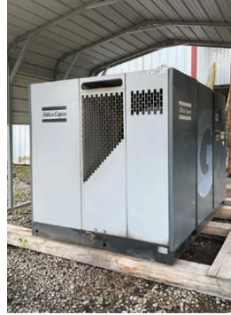
2014 Atlas Copco Air Compressor Model GA110. SN: APF 19206, 30' cord to breaker box, 45',600 PSI hose.
