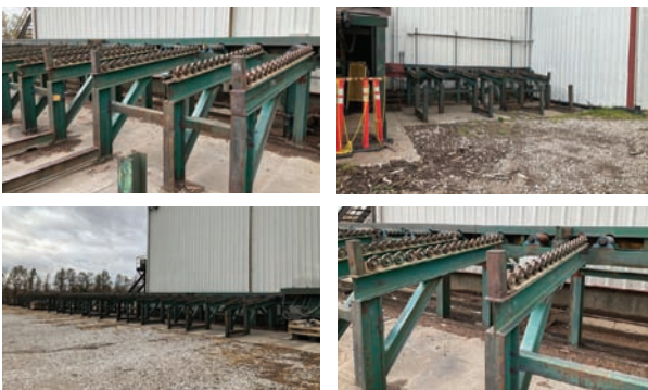
Salem Tie Sorting Line (Part of an entirety) 10 bunk sorting line, automatic sorting line, 135' overall.
