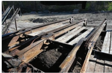
9193 $5,000.00 LOG DECK 3 strands, 12' wide x 23' long, H-78 chain, electric drive, working condition 260-633-4047
