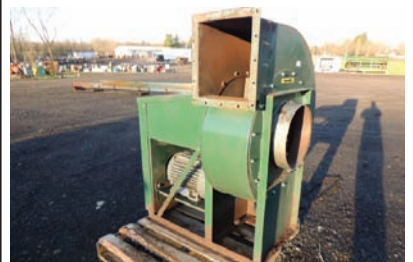
10359 BLOWER $2,500.00 36" dia dust blower, 20 hp electric powered, 14" inlet- 12"x15" outlet, excellent condition 260-633-4047
