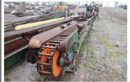
9063 $14,300.00 LOG TROUGH 30' long, 12" wide ladderback chain, electric gear box drive, 1 set of log kickers, good condition 260-633-4047
