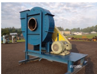
10366 DUST BLOWER $5,200.00 IAP dust blower, 24" dia inlet- 24" dia outlet, 150 hp electric drive, 18,000 cfm's very good condition 260-633-4047
