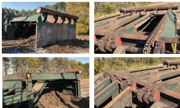
Log Deck Cylinders: Hydraulic. # of Strands: 5. Drive Type: Electric. Size: 14' x 16'. Stop'n'Load: no. Features and Notes: Heavy Log deck, 3/4" steel plate along front.
