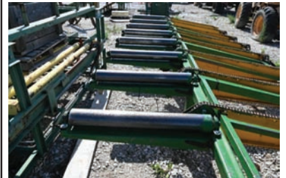
9204 $2,500.00 ROLL CASE roll case/ transfer deck, rollers are 30" wide x 19' long, transfer is 52" wide, electric drive, lighter duty and in good condition 260-633-4047
