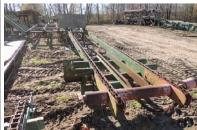
9096 TRANSFER DECK $4,250.00 2 strand transfer deck, 3' wide x 25' long, electric drive, 81X chain, good condition 260-633-4047
