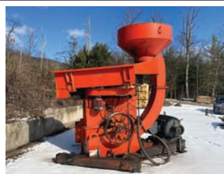
7603 $18,000 48" MORBARK CHIP PAC Heavy-Duty Chipper & Shaker Combo – Excellent Condition! Chipper: 3-knife design, powered by a 100 HP electric motor. Shaker: Driven by a 3 HP electric motor. All in very good working condition. Ready to go. 307-272-6738
