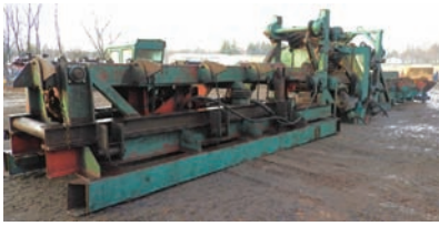
6047 DEBARKER $55,000.00 30" Cambio 5 arm ring debarker, electric drive, includes infeed/ outfeed log troughs and all controls, in good condition and ready for production 260-633-4047 Wolcottville, IN
