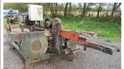
3099 $8,500.00 SINGLE HEAD RESAW Morgan single head resaw, has return belt, electric drive, good working condition 260-633-4047 Wolcottville, IN
