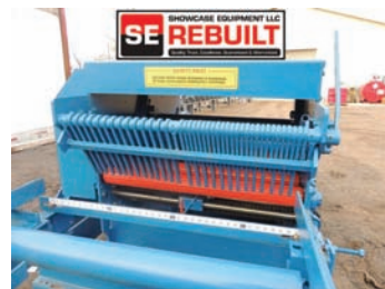
5112 $45,000.00 SHOWCASE REBUILT CORNELL GANG EDGER 6" x 36" capacity, 8' infeed/4' live outfeed, 1 movable & 1 stationary blade, this unit is completely rebuilt and ready for production, comes with a 6 month warranty , LIKE NEW CONDITION 260-633-4047
