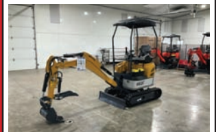
Unused IRE20 Mini Excavator — Specification & Features — Powered by a Yanmar 3TNV74F Engine. Bucket Capacity: 0.033. Rated Power/Speed: 17.2 kW / 3000 rpm. Horsepower: 18.4 HP. Fuel Type: Diesel. Displacement: 0.854 L. Fuel Capacity: 15 L. Track Width: 7". Maximum Unloading Height: 71". Maximum Excavation Depth: 67". Overall Machine Size: 115" x 44" x 96". — Contact — Specialist: Myron Miller, 574-536-6306.
