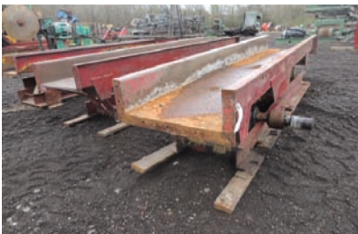
9236 VIBRATING CONVEYOR $10,500.00 30' L, hyd drive, 24" pan, 8" sides, 19" from floor to bottom of pan, good condition 260-633-4047
