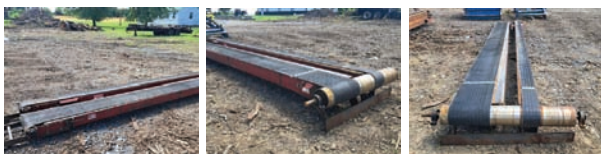
Mellot Tailing Belt Conveyor — Specifications & Features — Drive Type: None. Length: 16'. Overall Width: 30". Belt Width: 14" and 6". — Contact — Specialist: Daniel S, 717-406-9611.
