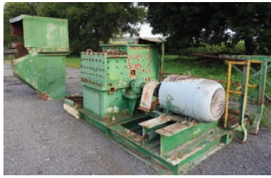
7155 WASTE GRINDER $8,500.00 Progress waste grinder, swinging hammer style, 125 hp electric drive, 1185 rpm's, unit needs to have hammers installed, good overall condition 260-633-4047 Wolcottville, IN
