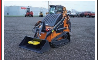
New Land Hero PLD-BC380 Mini Track Skid Steer Loader — Specification & Features — Powered by a 23 hp air-cooled gas engine. Hydrostatic drive controlled by joystick. Equipped with 40" quick coupler bucket. Includes auxiliary hydraulics. Lift capacity: 850 lbs. Equipped with 7" rubber tracks. Hydraulic cooler and fan included. — Description — Unused mini skid steer track loader with ride on platform. — Specialist — Myron Miller with any questions 574-536-6306
