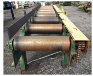
9251 ROLL CASE $8,500.00 30" wide x 21' long, 8" dia rolls, this unit is heavy duty and in very good condition 260-633-4047
