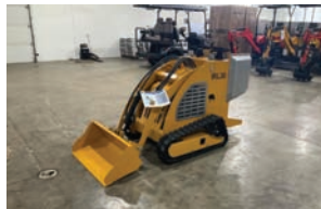
Unused IRL30 Mini Skid Steer — Specification & Features — Machine operating weight: 1322lb. Bucket Capacity: 0.153. Travel Speed (Low/High): 0-3.7 mph. Climbing Ability: 25%. Maximum Lifting Force: 400 lb. Maximum Working Height: 92". Maximum Pin Height: 70". Maximum Unloading Height: 66". Ground Clearance: 5". Bucket Dumping Angle: 30°. Bucket Width: 36". Overall Length: 86". Overall Width: 39". Carriage Width: 24". — Contact — Specialist: Myron Miller, 574-536-6306.
