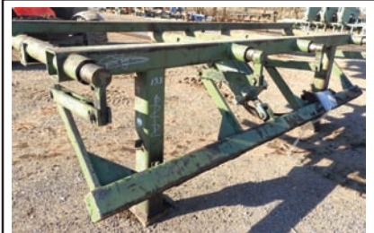
9244 CANT CATCHER $8,000.00 Reckart cant catcher for drop use with a drop belt, air powered, 4 arms, travel is 30", good working condition 260-633-4047
