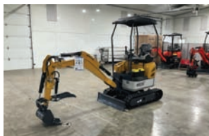
Unused IRE20 Mini Excavator — Specification & Features — Powered by a Yanmar 3TNV74F Engine. Bucket Capacity: 0.033. Rated Power/Speed: 17.2 kW / 3000 rpm. Horsepower: 18.4 HP. Fuel Type: Diesel. Displacement: 0.854 L. Fuel Capacity: 15 L. Track Width: 7". Maximum Unloading Height: 71". Maximum Excavation Depth: 67". Overall Machine Size: 115" x 44" x 96". — Contact — Specialist: Myron Miller, 574-536-6306.
