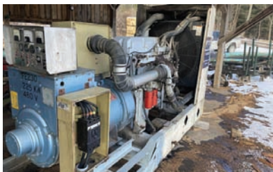
12610 $15,500 60 SERIES DETROIT GENSET 225 KW Generator Excellent Condition. 3 Phase / 338 Amps, 5487 Hours, 490 HP. Clean, powerful unit — ready to run. 307-272-6738
