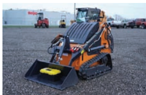
New Land Hero PLD-BC380 Mini Track Skid Steer Loader — Specification & Features — Powered by a 23 hp air-cooled gas engine. Hydrostatic drive controlled by joystick. Equipped with 40" quick coupler bucket. Includes auxiliary hydraulics. Lift capacity: 850 lbs. Equipped with 7" rubber tracks. Hydraulic cooler and fan included. — Description — Unused mini skid steer track loader with ride on platform. — Specialist — Myron Miller with any questions 574-536-6306
