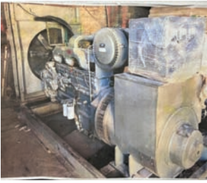
12617 $18,500.00 855 CUMMINS GENERATOR Fully rebuilt by Motive Engines in NY. Zero hours—never used. 277/480 volts, 12-wire setup can be configured for 208/480. Load bank tested at 362 amps. This is a solid gen-set. Best offer. 917-731-7439 Corona, NY.
