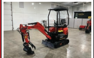
Unused TPM-16 Mini Hydraulic Excavator — Specification & Features — Engine: Briggs & Stratton 420cc 13.5 HP gasoline. Auxiliary hydraulic pilot guide control system. Transmission: Hydrostatic. 15-inch dig bucket with 3 teeth and 2 side bits. Hydraulic thumb. With rear counterweight. LED work lights. 40-inch push blade. Inverted boom (Kubota type). Tool box. 7-inch width rubber tracks. Four-post rollover protection canopy. With heat radiator. — Contact — Specialist: Myron Miller, 574-536-6306.
