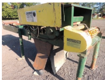
5118 $11,500.00 EDGER 4" x 30" wide capacity, 2 movable blades, includes BRAND NEW ARBOR, very good condition 260-633-4047
