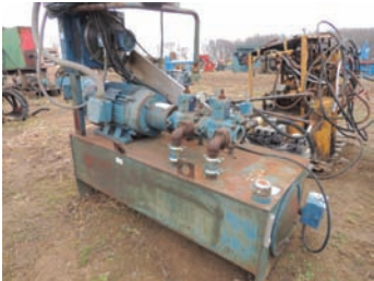
18186 HYDRAULIC PACK $5,000.00 30 HP electric motor w/double pump direct mounter, approx. 100 gal tank, lots of electric control valves, oil cooler, electric control box 260-633-4047
