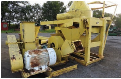
7154 CHIP-PAC $22,500.00 Fulghum 48" dia chipper, 3 knives, 150 hp electric drive, 5' x 5' shaker screen-electric drive, chip blower-electric drive, complete unit that is in good condition and ready to work 260-633-4047 Wolcottville, IN
