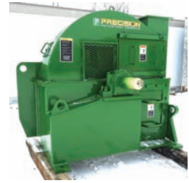
7159 CHIPPER $81,247.00 Precision 58" dia, 6 knife, hard surfaced anvils, Kwik-Change knife system, THIS UNIT IS BRAND NEW!! in-stock and ready to ship 260-633-4047 Wolcottville, IN
