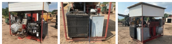
Deutz Power Unit with Hydraulic Pump and Air Compressor — Specifications & Features — Make: Deutz. Model: CD 2012L04 2V. Serial #: 11221896. Engine Cylinder: 4. Fuel: Diesel. Meter Reads: na. Horsepower: 100. Voltage: 12. Clutch: no. — Seller Statement — Liquid cooled motor, Parker pressure compensated Hyd pump, Model: P2075R001C25PA0081G1P SN: 11, 40 gpm, on slide, Hyd oil tank, fuel tank, Ingersol Rand air compressor model 15T-T3020TM on tank starts with air clutch, Portable unit, needs pulley on motor, everything is in good working condition. — Contact — Specialist: Daniel S, 717-406-9611.
