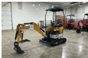
Unused IRE20 Mini Excavator — Specification & Features — Powered by a Yanmar 3TNV74F Engine. Bucket Capacity: 0.033. Rated Power/Speed: 17.2 kW / 3000 rpm. Horsepower: 18.4 HP. Fuel Type: Diesel. Displacement: 0.854 L. Fuel Capacity: 15 L. Track Width: 7". Maximum Unloading Height: 71". Maximum Excavation Depth: 67". Overall Machine Size: 115" x 44" x 96". — Contact — Specialist: Myron Miller, 574-536-6306.
