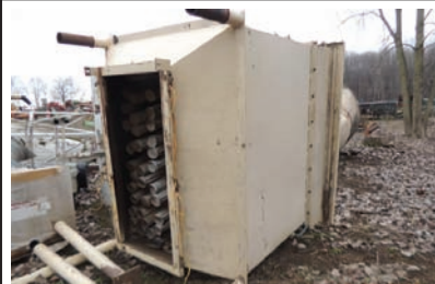
10309 BAG HOUSE SYSTEM $4,000.00 Honeyville Metal baghouse is approx. 8' x 8', 72 - 5" x 60" bags, 11" x 13" inlet, 28" x 63" bottom outlet, includes blower and numerous pipes, good condition 260-633-4047
