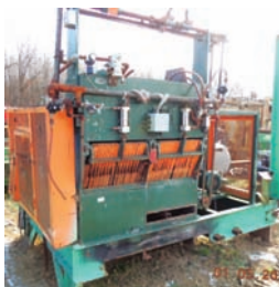
4026 CORLEY GANG EDGER 8" capacity, includes infeed/outfeed, electric drive, THIS UNIT NEEDS TO BE REBUILT, CALL FOR OPTIONS!! 260-633-4047
