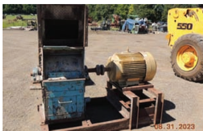
7134 $6,300.00 WASTE GRINDER Roberts hammer mill/ waste grinder, top feed, 60 hp electric drive, 3600 rpm's, good working condition 260-633-4047
