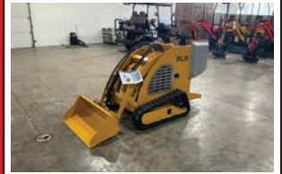
Unused IRL30 Mini Skid Steer — Specification & Features — Machine operating weight: 1322lb. Bucket Capacity: 0.153. Travel Speed (Low/High): 0-3.7 mph. Climbing Ability: 25%. Maximum Lifting Force: 400 lb. Maximum Working Height: 92". Maximum Pin Height: 70". Maximum Unloading Height: 66". Ground Clearance: 5". Bucket Dumping Angle: 30°. Bucket Width: 36". Overall Length: 86". Overall Width: 39". Carriage Width: 24". — Contact — Specialist: Myron Miller, 574-536-6306.
