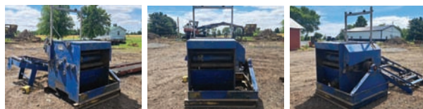
Cornell Edger — Specifications & Features — Year: unknown. Make: Cornell. Model: unknown. Serial #: SE254470. Drive Type: Line-Shaft. # of Blades: 2. # of Moveable Blades: 1. # of Stationary Blades: 1. Blade Type: Circle. Cut Capacity: 6"x36". Infeed Measurement: 38". Outfeed Measurement: 38". Arbor Size: 2 1/4". Lasers: no. Edger Set Up: Portable. — Seller Statement — Has air foot pedal, 40"x8' roll case included — Contact — Specialist: Daniel S, 717-406-9611.
