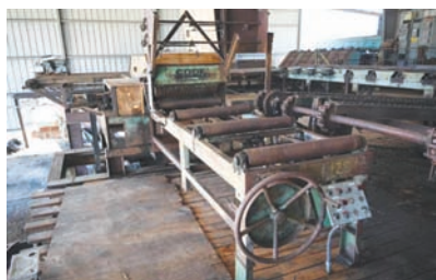
5114 $10,750.00 COOK EDGER Model:36EZTD, SN: 42, 5" x 21' tailing belt outfeed, 38" x 9' infeed rolls, 6" x 36" infeed cap, control panel, manual blade set, (2) 20" blades both are adjustable, electric drive, good heavy duty older unit 260-633-4047
