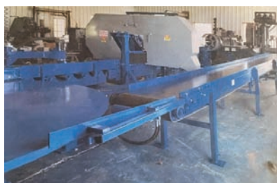
3612 $80,000.00 2023 HERSHBERGER MFG. STAVE RESAW 21" sq. capacity, line shaft hook-up, hyd. variable speed conveyor belts, hyd unit is included. 36" band wheel with hyd tension, 2" bands x 20' 1". Could be Converted to a Grade Resaw. This outfit is same as NEW! 812-718-5997
