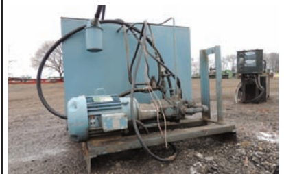
18206 HYD UNIT $3,100.00 10 hp electric drive, approx 160 gal tank, pressure comp pump, good working condition 260-633-4047
