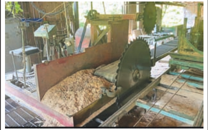
2612 $38,000.00 COMPLETE FRICKCO CIRCLE MILL Mellott log deck with stop and unloader, #5 turner, track and hydraulic drive. Features a 4-dog carriage with air dogs and drive, electric networks, and husk with 56" blade, top saw, and slab belt. Includes pulleys and belts, Frick 2-saw edger with roll case, plus a 150 HP motor and starter. A complete mill package. 330-603-5365 Doylestown, OH.
