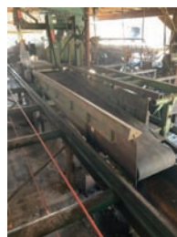
9243 DROP BELT CONVEYOR $7,200.00 Reckart drop belt, 24" wide x 13' long, air cylinder for up-down, hyd drive, good working condition 260-633-4047
