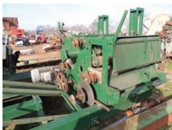
5103 $85,000.00 TIERNEY GANG SAW/EDGER 6" capacity gang edger, gang side is 16" wide- edger side is 28" wide, this unit will be "SHOWCASE REBUILT" and come with a full warranty, call to customize to your specs and for a time-line 260-633-4047
