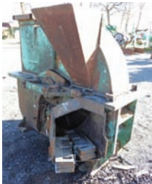
7161 CHIPPER $12,500.00 PHL Industries 48" dia chipper, 6 knife wheel with 3 blocked, includes some spare knives, good working condition 260-633-4047 Wolcottville, IN
