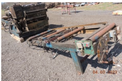
5111 $17,250.00 CORNELL EDGER 6" x 42" capacity, MN: HE42, SN: 703-10-81, single arbor, (4) 19" saws, 2 movable blades, 8" infeed, 8' powered outfeed, electric drive, comes w/ spare spacers, saws and laser lights 260-633-4047
