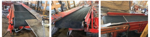
Slab Drop Belt — Specifications & Features — Make: NA. Drive Type: Hydraulic. Up & Down Cylinder: Air. Length: 154". Overall Height: Sloped from 31" to 40". Overall Length: 147". Overall Width: 4'. Belt Width: 32". — Seller Statement — Very good condition
