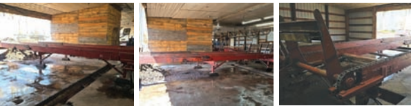
Mellot Log Deck — Specifications & Features — Make: Mellot. Drive Type: Hydraulic. Up & Down Cylinder: Hydraulic. # of Strands: 3. Stop'n'Load: yes. Size: 10'x31' 3"x41 1/2". Chain Type: Ladderback Chain. — Seller Statement — 36" loading arms, two decks jointed to make one.
