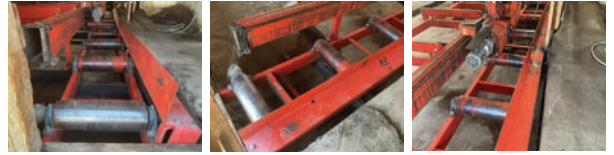
Shop-Built Live Roll Case — Specifications & Features — Make: Shop-built. Drive Type: Hydraulic. Roller Size: 6.5" x 20". Overall Dimensions: 30" x 30'. Shaft Size: 1 3/4". — Seller Statement — Behind mill to take off long stock
