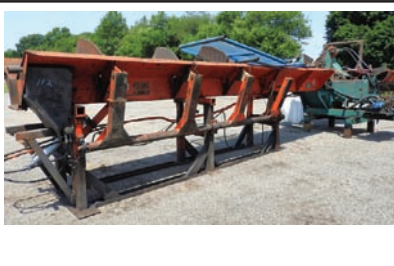
6051 $35,000.00 DEBARKER Morbark 640 debark complete line, includes infeed/ outfeed troughs, operating cab and all controls, this unit is set up to run with all hydraulics, complete and ready for production 260-633-4047
