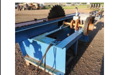
2094 $5,000.00 SPLITTER SAW designed to split cants, boards, etc., 50hp electric drive, 81x chain, 40" dia inserted tooth blade, hyd drive on feed, good working condition 260-633-4047 Wolcottville, IN
