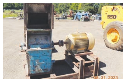
7134 $6,300.00 WASTE GRINDER Roberts hammer mill/ waste grinder, 1/4" screen, top feed, 60 hp electric drive, 3600 rpm's, good working condition 260-633-4047
