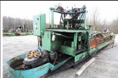
6048 $29,500.00 DEBARKER Precision rosser head debarker, 36" capacity, electric drive on head, self-contained hyd unit for carriage etc., upgraded to chain drive for carriage, has flat barn sweep underneath, working condition 260-633-4047
