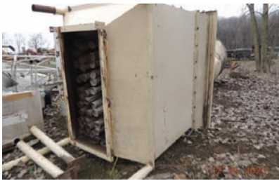
10309 $4,000.00 BAG HOUSE SYSTEM Honeyville Metal baghouse is approx. 8' x 8', 72 - 5" x 60" bags, 11" x 13" inlet, 28" x 63" bottom outlet, includes blower and numerous pipes, good condition 260-633-4047
