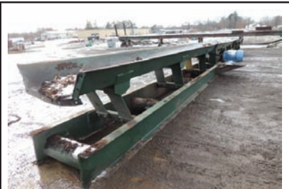
9119 $13,750.00 VIBRATING CONVEYOR Jeffrey vibrating conveyor, 18" wide pan x 36' long, 6" tall sides, electric drive, good working condition 260-633-4047
