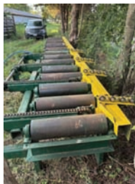
9303 ROLL CASE $7,500.00 24" wide x 20' long, 2 strand pop-up transfer, transfer goes both directions, hyd drive, heavy duty and in excellent condition, ready for production 260-633-4047
