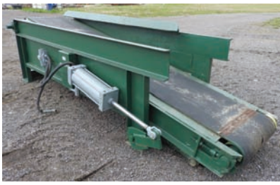
9292 SLAB DROP BELT $6,500.00 24" wide x 10' long, built for left-hand mill, air cylinder for up-down motion, good working condition 260-633-4047
