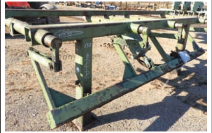
9244 $8,000.00 CANT CATCHER Reckart cant catcher for drop use with a drop belt, air powered, 4 arms, travel is 30", good working condition 260-633-4047
