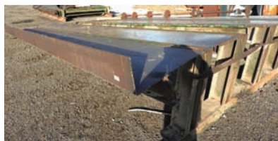
9253 $8,500.00 TRANSFER DECK 5 strand heavy duty deck, 12' 6" wide x 25' long, electric drive, H-78 chain, very good condition 260-633-4047
