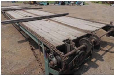
9091 $14,300.00 GREEN CHAIN 3 strand, 9'6" wide x 101' long, electric drive, 8X chain, good condition 260-633-4047 Wolcottville, IN
