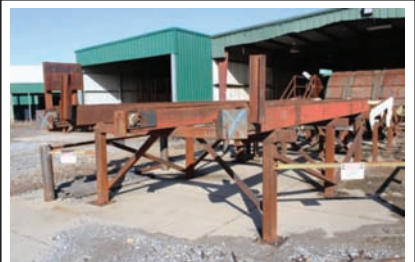
9266 $5,750.00 TRANSFER DECK 3 strand transfer deck, 10' wide x 18' long, 5 hp electric gear-box drive, 81X chain, good working condition 260-633-4047
