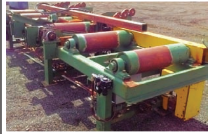
9281 $5,500.00 ROLLCASE rollcase/ pop-up transfer, 30" wide x 13' long, 3 strand transfer, hyd and electric drive, has cant flippers, heavy duty and in excellent condition 260-633-4047
