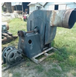
10608 $2400 STURTEVAT WESTINGHOUSE INDUSTRIAL BLOWER 6-paddle unit with 48" diameter and 16" inlets/outlets. Model size 717, Style W63694. Powered by a 20 HP, 3-phase electric motor. Ideal for handling dust or wood chips. In good working condition. 417-737-9850
