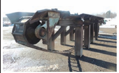
9090 $14,300.00 LOG TROUGH 40' long, 110 ladder-back chain, 14" wide, s-style drive, no power, good working condition 260-633-4047 Wolcottville, IN
