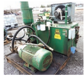
18240 HYD POWER UNIT $4,500.00 40hp electric drive hyd unit, pressure comp pump, approx. 150 gal reservoir, includes cooling radiator and accumulator, very good condition 260-633-4047
