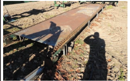
9095 $5,000.00 TRANSFER DECK 2 strand transfer deck, 5' wide x 23' long, 81XH chain, BRAND NEW DRIVE SHAFT/ SPROCKETS, very good condition 260-633-4047 Wolcottville, IN
