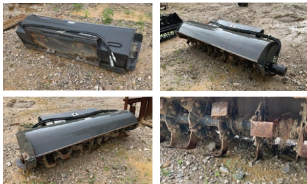
6' Tiller — Description — Skid steer quick attach, hyd. powered
