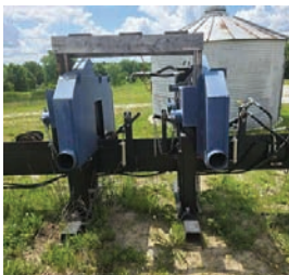
3616 TRU CUT DOUBLE HEAD RESAW $12,000.00 Hydraulic motor for power, air-operated up and down movement, hold-down wheel, and hydraulic motor on the feed belt. In good condition. 574-536-1646 Brashear, MO.
