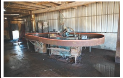
15078 $7,400.00 BAND SAW SHARPENER Armstrong, Model #6 RH, SN: 16154, electric drive, includes extra grinding wheels and all clamps and strands, Armstrong #58-B filling clamp, working condition 260-633-4047 Wolcottville, IN
