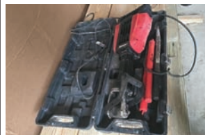
Bauer Electric Jackhammer — Description — 35 pound hammer, Serial No. 370452207
