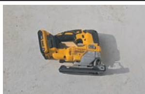
DeWalt Cordless Variable Speed Jigsaw — Description — Model No. DCS334, Brushless, Does not include blade, Includes 2 amp battery, Tilttable table
