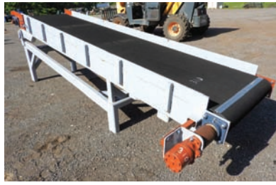
9298 DROP BELT $12,500.00 slab drop belt, 34" wide x 12' long, hyd drive, hyd cylinder for up-down movement, brand new and ready for production 260-633-4047
