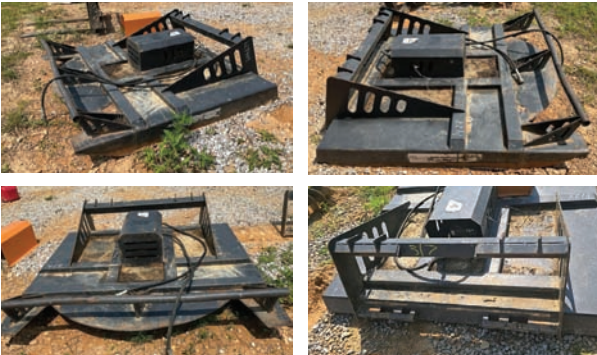
Brush Hog Attachment — Description — 70"x70" brush hog attachment, unknown make and model, Gearbox leaking at the bottom, Brush hog is mainly for parts
