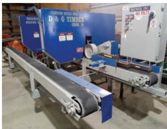
3601 BREWER 2 HEAD RESAW $18,500.00 3-phase, 480V electric-powered unit with 30" band wheels, air strain, and return belt. This is a reconditioned unit, measuring 7' wide by 13'9" long. Just connect the wires—she's ready to run. 260-740-8036 Spencerville, IN.
