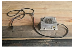
Intelligent Charger — Description — Model: H82-36V15A, Input: 110-245VAC 45- 65Hz, Battery: LiPo4 12 cells, Cord is loose
