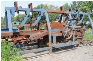
19008 SCRAGG MILL $86,250.00 Fast Line scragg mill, similar to "Big Jake", twin blades 56" dia, electric drive, includes off-bearer belts, price includes controls and machine gone through shop, ready for production 260-633-4047
