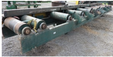
9301 ROLL CASE $7,500.00 34" overall width, 8-1/2" x 24" rollers x 23' long, includes hyd powered kickers, hyd drive, heavy duty and in excellent condition 260-633-4047
