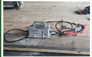
Intelligent Charger — Description — Model: H82-36V15A, Input: 110-245VAC 45-65 Hz, Battery: LiFePo4 12 cells
