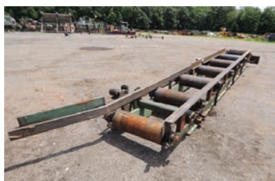
9192 $3,500.00 ROLL CASE 24" wide x 19' long, 81/2" dia rollers, hyd drive, heavy duty and in good working condition 260-633-4047
