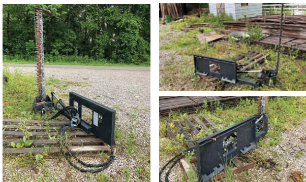
Sickle Bar Mower — Description — Model SBM-12-72-W. SN: ZW-01703. 6' bar, hyd drive, skid steer quick attach mounted, bar holding shaft has slight bend. Remote controls for bar lift.
