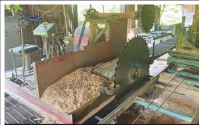
2612 COMPLETE FRICKCO CIRCLE MILL $38,000 Mellott log deck with stop and unloader, #5 turner, track and hydraulic drive. Features a 4-dog carriage with air dogs and drive, electric setworks, and husk with 56" blade, top saw, and slab belt. Includes pulleys and belts, Frick 2-saw edger with roll case, plus a 150 HP motor and starter. A complete mill package. 330-603-5365
