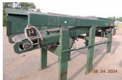
9191 $9,500.00 DROP BELT Pendu slab drop belt, 24" wide x 10' 6" long, hyd drive, twin air cylinders for up-down on belt, heavy duty and in excellent condition 260-633-4047
