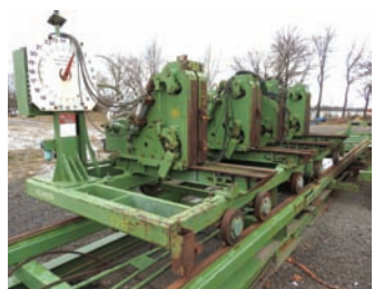
2096 $45,000.00 HMC CIRCLE MILL HMC 4 head-block circle mill, complete mill package, includes husk w/ top saw, carriage drive, operator cab, and all controls, price includes BRAND NEW set-works and mill gone through shop and ready for production 260-633-4047 Wolcottville, IN
