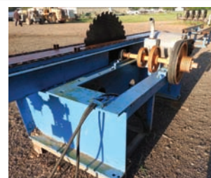
2094 $5,000.00 SPLITTER SAW designed to split cants, boards, etc., 50hp electric drive, 81x chain, 40" dia inserted tooth blade, hyd drive on feed, good working condition 260-633-4047 Wolcottville, IN
