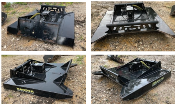
Skid Steer Brush Hog — Description — Quick attach, 78" brush hog attachment, hyd. powered
