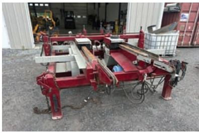
14608 $22,000.00 KEYSTONE DOUBLE HEAD NOTCHER Pallet stringer notcher in great working condition with 30 HP motors. Handles material from 28" to 72". 434-270-4851 Long Island, VA
