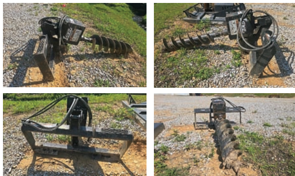
Lowe Auger Attachment — Description — Auger: 10" wide. Hydraulic hose
