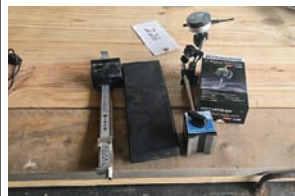
Digital Indicators and Calipers — Description — Pittsburgh 1" Digital Indicator: Mounted on magnetic base, Pittsburgh 6" digital caliper, Wixey Digital Readout
