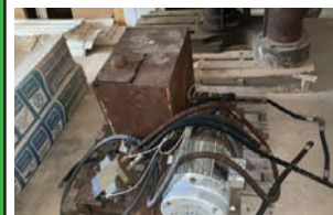
Hydraulic Pack — Description — 5 hp electric motor, 18" x 16" x 12" tank, solenoid valve
