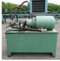
18246 HY POWER UNIT $3,500.00 40 hp electric, vane type pump, includes cooling radiator, approx. 120 gallon capacity, good working condition 260-633-4047
