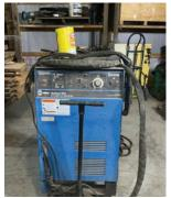
Miller Spectrum Plasma Cutter - Specifications & Features — Make: Miller. Model: Spectrum 1000. Serial #: KG167221. — Seller Statement — 230/460/575v. 3 phase, 70 psi. Air, electric cord not included, good condition — Location –
