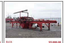
**EDGER** Meadows edger 4" thick x 36" wide capacity, infeed/ outfeed, 1 movable-1 stationary blade, includes BRAND NEW blades and collars, comes with sawdust blower, recently in production and in good working condition
