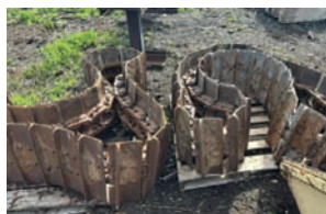
Cat D5 John Deere 750 Tracks — Description — 40 links 20" wide
