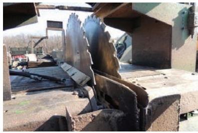
19009 SCRAGG MILL $69,500.00 Industries PHL log length scragg mill, 48" dia. blades, electric drive, 2 slab drop belts, all electrical and controls included, this machine was recently in production and is in very good condition 260-633-4047 Wolcottville, IN
