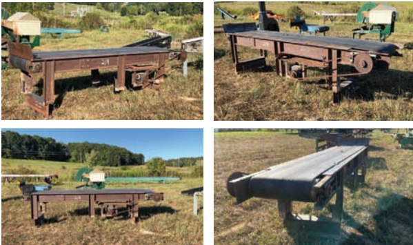
Belt Conveyor — Specifications & Features — Drive Type: Line-Shaft. Length: 12'. Overall Height: 36". Overall Width: 32". Belt Width: 23". — Seller Statement — Heavy duty build
