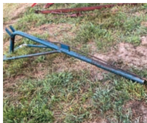
King Kutter 3 Pt. Slip Scoop — Description — 30" x 30" bucket, push or pull type
