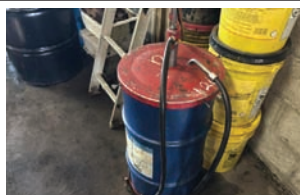
Hand Gear Oil Pump on Wheels — Description — 120lb
