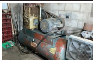
Quincy Air Compressor — Specifications & Features — Make: Quincy. Serial #: 702829LS. — Seller Statement — Powered by 20 HP Lincoln Electric Motor, Tank: 21"x66",
