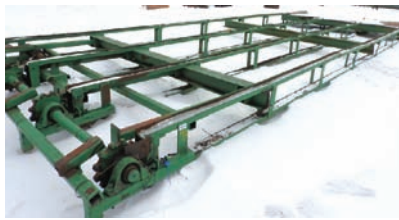
9272 TRANSFER DECK $7,500.00 4 strand transfer deck, 10' wide x 27' long, PRICE INCLUDES BRAND NEW 81X CHAIN, good condition 260-633-4047
