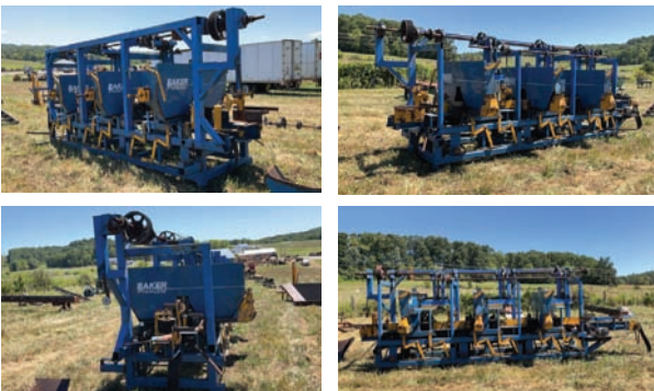
Baker Band Resaw — Specifications & Features — Make: Baker. Model: BBR-3 Head. Serial #: na. Drive Type: Line-Shaft. # of Heads: 3. Return: no. Blade Size: 1". Blade Tension: Manual. Cut Capacity: t6" x 10". Overall Dimensions: 7' x 21' x 92" tall. Wheel Size: 3/4" x 28". Guide Type: Roller. — Seller Statement — Feed rolls are mechanically driven, everything runs by line shaft. Includes cant sizer on end.
