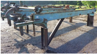
9293 $8,500.00 LOG DECK HMC 3 strand log deck, H-78 chain, stop-load for debarker, 10' 6" wide x 19' long, Tulsa Winch electric drive, very good condition 260-633-4047
