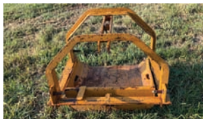
King Kutter 3 Pt. Slip Scoop — Description — 30" x 30" bucket, push or pull type
