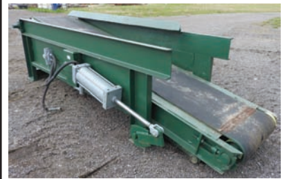
9292 $6,500.00 SLAB DROP BELT 24" wide x 10' long, built for left-hand mill, air cylinder for up-down motion, good working condition 260-633-4047
