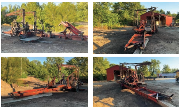
Meadows # 1 Sawmills — Specifications & Features — Make: Meadows. Model: #1. Serial #: n. Power: no. Hitch Type: pin. # of Headblocks: 3. Modular Mill Type: Hydraulic. Blade Size on Husk: 48". Overall Dimensions: 8'6" x 34' x 10' tall,. Setworks: no. Tire Size: 7.00-15. Automated: yes. Carriage Dimensions: 4' x13'. Log Turner: no. — Seller Statement — 25 topsaw, hyd set, hyd feed, panagraph, tires are flat, 38' track, 22" x 6' offbear belt,
