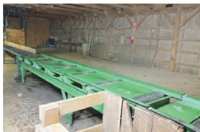
9284 ROLL CASE $3,500.00 live roll case 24" wide x 15' long, electric drive, 6 1/2" dia rolls, good working condition 260-633-4047
