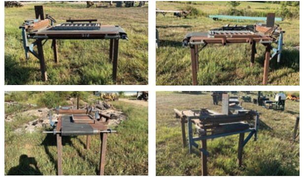
Side Transfer Belt and Deadroll — Description — Size: 65"x35"x40 1/2", Belt width: 20 3/8", Deadroll: 40"x18"
