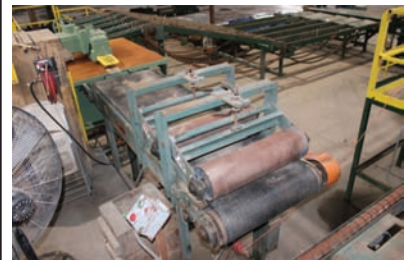
9317 BELT CONVEYOR $2,500.00 24" wide x 9' long, approx 4" tall sides, electric drive, has 2 pinch rollers on drive end, very good condition 260-633-4047
