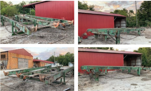
Log Deck — Specifications & Features — Make: na. Drive Type: Electric. Up & Down Cylinder: Hydraulic. # of Strands: 3. Stop'n'Load: yes. Size: 13'8" x 28". Chain Type: WH-124.
