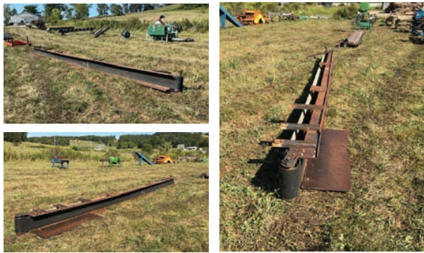
Belt Conveyor — Specifications & Features — Drive Type: None. Length: 27' 5". Overall Height: 20", includes one 36" leg. Overall Width: 14 1/2". Belt Width: 11".
