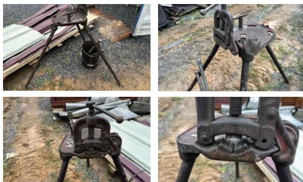
Pipe Threader — Description — Ridgid, stand, No40, 8 dies, 1/2" to 1 1/2" — Location — 238 B Old Leacock Rd, Gordonville, PA 17529. Eligible For Free Loadout
