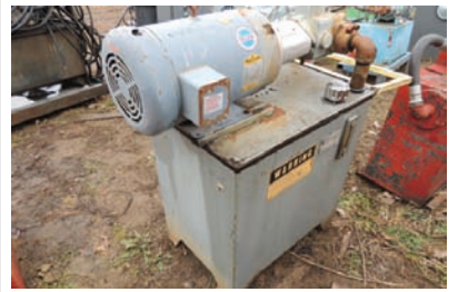
18121 $2,850.00 HYD. UNIT 10 hp hydraulic power pack, 40 gal. tank, pump Model PVR15-15B15-RF-0-5-A-1, good condition 260-633-4047
