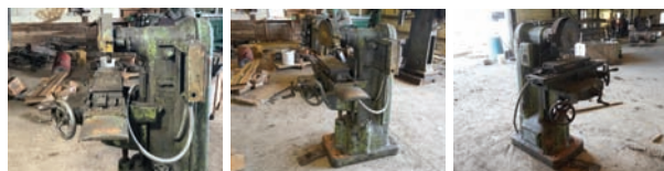
Covell Surface Grinder — Description — 6" x 18" magnetic table
