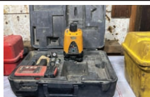
Laser Level — Description — LD400 detector, Works, needs recalibrated
