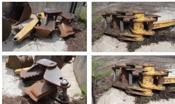
Stump Splitter — Description — For use on excavator, 28" jaws. Mechanical stump splitter, fits John Deere and Hitachi 270 excavators
