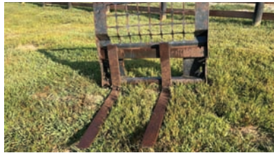
Skid Steer Forks — Description — 4" x 42" forks, quick attach, fork holding rail is broken
