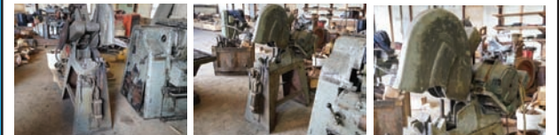
DoAll Metal Chopsaw — Description — 14" abrasive blades, 7.5 hp electric motor
