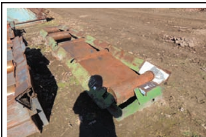
9147 ROLL CASE $3,500.00 24" wide x 15' long, 8" dia rolls, good working condition 260-633-4047
