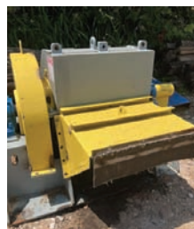
7612 $37,000.00 MONTGOMERY HOG Horizontal feed. This machine has been fully serviced with new anvils, bolts, and holders, and includes a chute underneath. It is in very good working condition. A right-hand heavy gearbox is also available as an additional option. 270-750-1054 Irvinginton, KY
