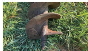
3 pt. Post Hold Digger — Description — 12" auger, PTO drive
