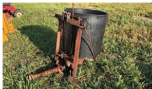
3 Pt Spreader — Description — Fertilizer spreader, PTO drive
