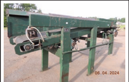
9191 DROP BELT $9,500.00 Pendul slab drop belt, 24" wide x 10' 6" long, hyd drive, twin air cylinders for up-down on belt, heavy duty and in excellent condition 260-633-4047
