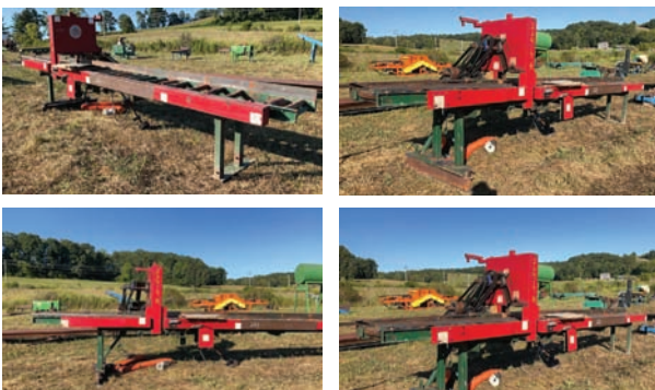
Morgan Chop Saw — Specifications & Features — Year: na. Make: Morgan. Model: manual. Serial #: no. Blade Size: 22". Blade Up/Down: manual. Cut Capacity: 6" x 12". Infeed: 24" x13' live Rollcase!. Outfeed: 24" x 70" live Rollcase with material stops. Overall Machine Measurement: 6' x 20' x 76".
