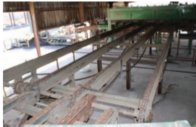
9268 $8,500.00 TRANSFER DECK 4 strand transfer deck, 10' 5" wide x 35' long, electric gear-box drive, 81X chain, good working condition 260-633-4047
