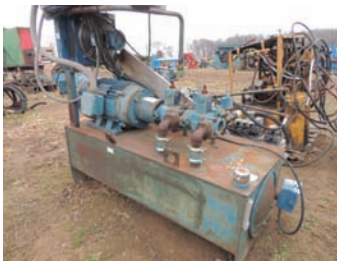
18186 HYDRAULIC PACK $5,000.00 30 HP electric motor w/double pump direct mounter, approx. 100 gal tank, lots of electric control valves, oil cooler, electric control box 260-633-4047
