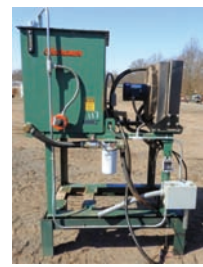
18244 HYD RESERVOIR $850.00 Hyd tank and cooler, approx 95 gal capacity, has cooling radiator and electric tank heater, very good condition 260-633-4047
