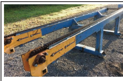
9216 TRANSFER DECK $2,500.00 2 strand transfer deck, 28" wide x 14' long, #80 roller chain, no drive, good condition 260-633-4047
