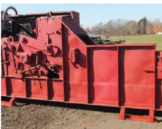
7611 $45,000.00 SB24E ROTO CHOPPER High-capacity waste grinder featuring a 24" wide infeed belt, 125 HP, electric drive. Well-maintained and in excellent working condition—ready to perform. 518-807-2779 Esperance, NY.
