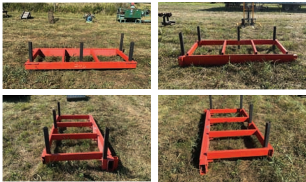
Bed Extension for Wood-Mizer Sawmill — Description — 107"x45"x12", Includes four 29" posts
