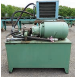
18246 HYD POWER UNIT $3,500.00 40 hp electric, vane type pump, includes cooling radiator, approx. 120 gallon capacity, good working condition 260-633-4047
