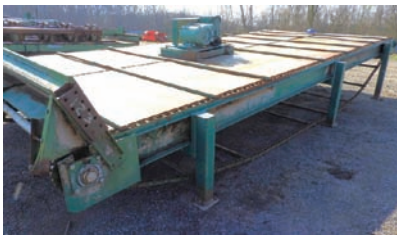
9290 $7,500.00 SLAB DRAG CONVEYOR slab drag waste conveyor, 10' 6" wide x 20' long, has steel slats to drag waste/ slabs, electric drive, good working condition 260-633-4047
