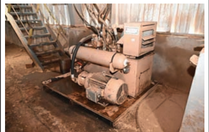
18199 HYD UNIT $4,300.00 40 hp electric, approx 150 gal capacity tank, PVR50 hyd pump, includes all valves attached, very good condition 260-633-4047
