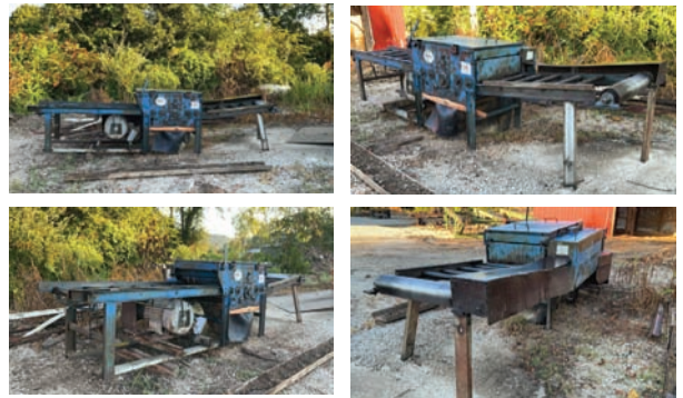
Cornell Edger — Specifications & Features — Year: na. Make: Cornell. Model: 3 Saw. Serial #: na. Drive Type: Electric. # of Blades: 3. # of Moveable Blades: 1. # of Stationary Blades: 2. Blade Type: Circle. Cut Capacity: 4" x 25". Infeed Measurement: 30" x 6". Outfeed Measurement: 30" x 5". Arbor Size: 2 7/16". Lasers: no. Edger Set Up: Stationary. — Seller Statement — 50 hp electric motor!
