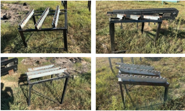
Dead Roll Table and Steel Frame — Description — 46"x41", Slopes from 41" to 30 1/2", Steel Frame: 32"x101"
