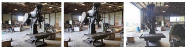
Baker # 314 Drill Press — Description — 16" stroke, automatic feed, 3 hp electric motor 1 phase,
