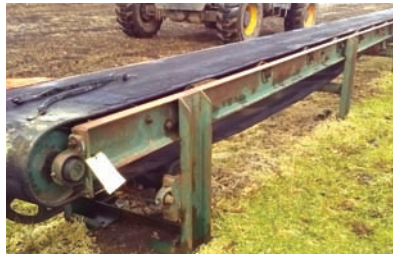
9279 BELT CONVEYOR $4,000.00 24" wide x 30' long, electric drive, good working condition 260-633-4047
