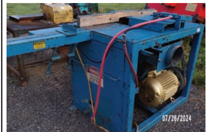
14079 $7,000.00 NOTCHER Brewer single head notcher, 15 hp electric drive motor, indexable head, good working condition 260-633-4047 Wolcottville, IN
