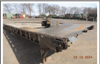
9169 GREEN CHAIN $5,250.00 2 strand green chain, 5' 6" wide x 32' long, gearbox drive, C-55 rooftop chain, good working condition 260-633-4047
