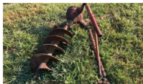
3 pt. Post Hold Digger — Description — 12" auger, PTO drive
