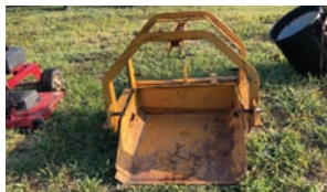
King Kutter 3 Pt. Slip Scoop — Description — 30" x 30" bucket, push or pull type
