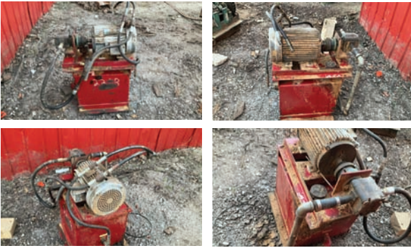
Hydraulic Pak — Description — 20" x 16" x 18" tank, 10 hp electric motor on pump
