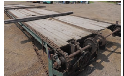
9091 $14,300.00 GREEN CHAIN 3 strand, 9'6" wide x 101' long, electric drive, 8X chain, good condition 260-633-4047
