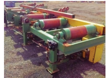
9281 ROLLCASE $5,500.00 rollcase/ pop-up transfer, 30" wide x 13' long, 3 strand transfer, hyd and electric drive, has cant flippers, heavy duty and in excellent condition 260-633-4047
