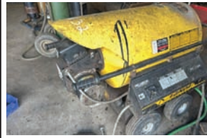
Landa Gold Series Steam Cleaner — Description — Portable Oil Burner, Model 7-00033, 4Gal a minute 2000 PSI, 220 Electric powered
