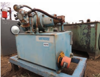
18218 HYD POWER UNIT $1,150.00 7 1/2 hp electric power, vane type pump, good condition 260-633-4047
