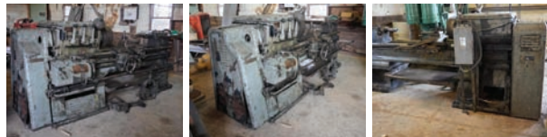
R & McDougall Engine Lathe — Description — 14"Swing, 48"bed, 2 steady rests working cond.
