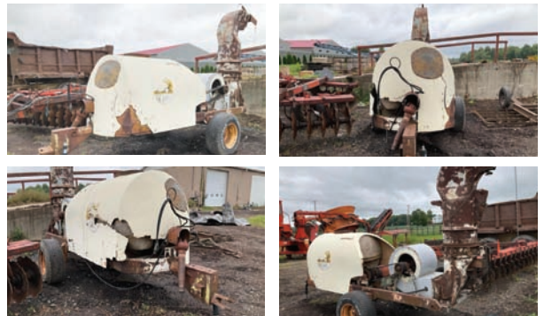
Crop Sprayer — Description — Pto drive, blower has no motor. Blower for fanning burning brush piles, set up to spray diesel fuel or liquid of choice.
