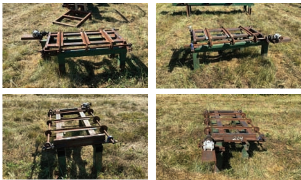
Side Transfer Deck — Specifications & Features — Make: na. # of Strands: 3. Overall Dimensions: 51"x36"x25".
