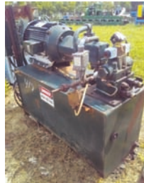
18247 HYD POWER UNIT $2,500.00 20 hp electric drive hyd power unit, gear style pump, approx 40 gal reservoir, includes control panel, good working condition 260-633-4047
