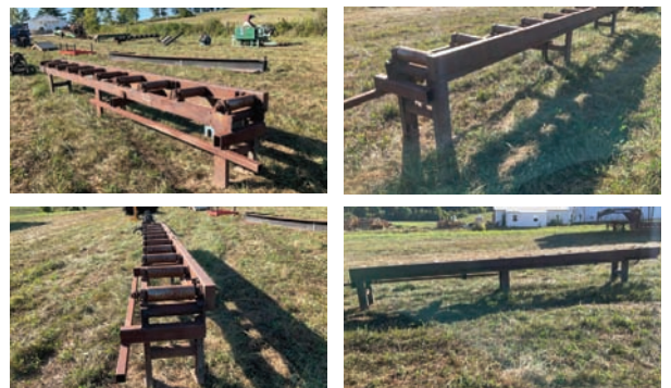
Live Rollcase — Specifications & Features — Make: na. Drive Type: None. Roller Size: 4" x 12". Overall Dimensions: 19" x 18'. Shaft Size: 1 1/4".
