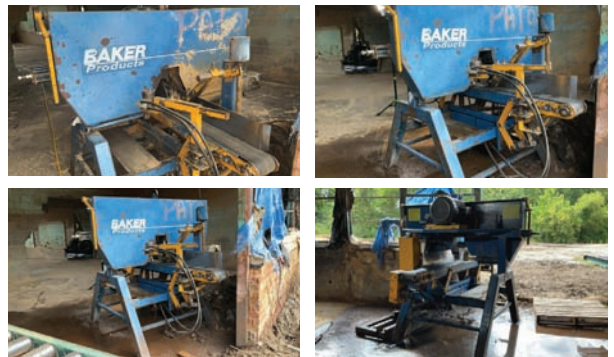
1996 Baker Band Resaw — Specifications & Features — Make: Baker. Model: BBR. Serial #: 96-1853. Drive Type: Electric. # of Heads: 1. Return: no. Blade Size: 1". Blade Tension: Manual. Cut Capacity: 6" x 12". Overall Dimensions: 6' x 7'. Wheel Size: 7/8" x 28". Guide Type: Roller. — Seller Statement — Hyd feed, self contained hyd unit, 20" blower, 20 hp motor on head,
