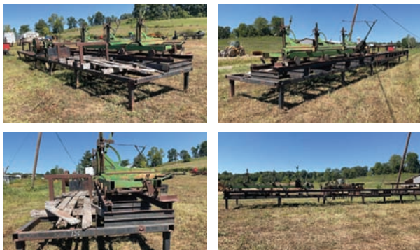
Frick Sawmill — Specifications & Features — Make: Frick. Model: na. Serial #: na. Manual: yes. # of Headblocks: 3. Overall Dimensions: 8' x 55' with mandrel removed. Log Deck: no. Log Turner: no. — Seller Statement — Stationary mill, manual carriage, 15' carriage
