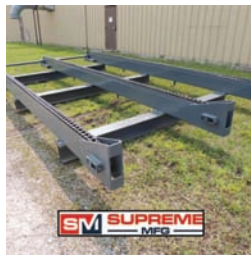
9085 $24,500.00 SUPREME MFG LOG DECK 3 strand 10' wide X 20' long log deck, Tulsa Winch electric drive, H-78 chain, heavy duty built, BRAND NEW! 260-633-4047
