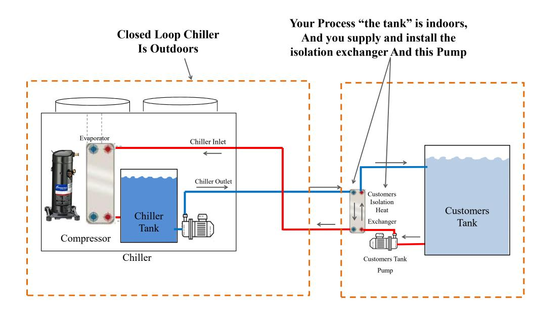
Standard Closed Loop Chiller Cooling a Customer's non-jacketed Tank, via an isolation exchanger and tank pump.
