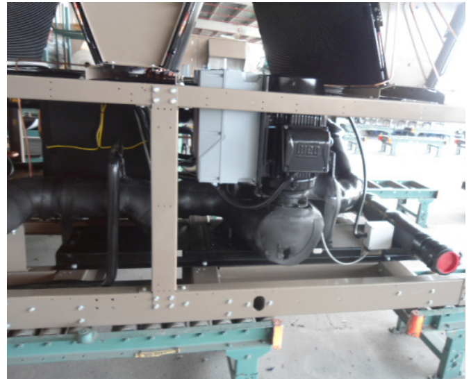
FIGURE 1 – TYPICAL HYDRONIC KIT COMPONENTS IN AN AIR-COOLED CHILLER (SHOWN WITH CONDENSER FAN REMOVED).
