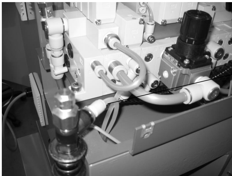
Fig. 7-3 Air supply to pressure plunger
