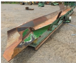
9295 VIBRATING CONVEYOR Webster vibrating conveyor, 18" wide pan x 25' long, electric drive, includes chipper feed spout, good working condition 260-633-4047
