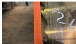
Double cut Bandsaw Blades — Description — 89 plate, VDP, 14 gauge, 2" space, 10 blades,
