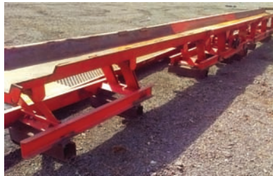
9282 VIBRATING CONVEYOR Morbark vibrating conveyor, 17" pan, 30' long, includes drive but no power, good condition 260-633-4047
