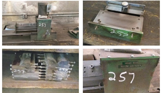
Guide Dressing Machine and Jig — Description — Setting jig, Includes 12" guide blocks
