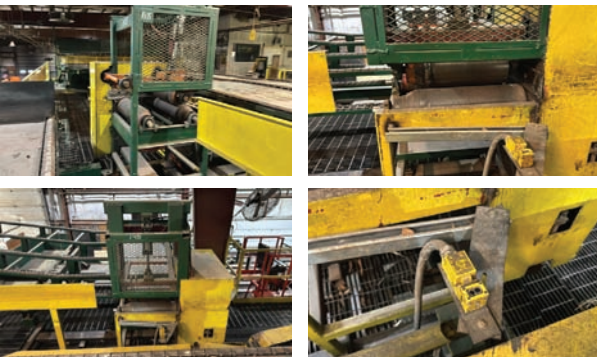
Board Side Transfer — Description — 23" bottom rollers, 18" hydraulic hold down roller, electric gearbox drive, board sensor
