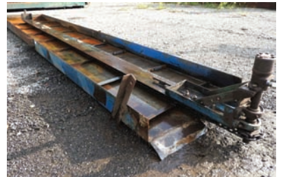
10383 $3,500.00 BARN SWEEP Cornell style chain, hyd drive, pan is 36" wide x 18' long, working condition 260-633-4047
