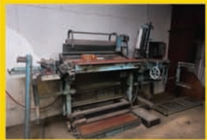
McDonough 6' Band Head Rig, 17 degree slant, Double Cut
