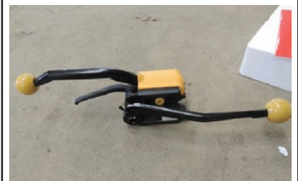
20298 $550.00 STRAPPING TOOL manual seal-less strapping tool for metal banding, similar to Fromm, will do banding from 1/2" up to 3/4" wide, BRAND NEW IN STOCK! 260-633-4047
