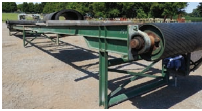
9305 BELT CONVEYOR $9,500.00 60" wide x 50' long, electric drive, no sides, good working condition 260-633-4047
