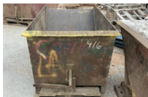
Self Dumping Hopper — Description — 36"x61"x30 1/2"
