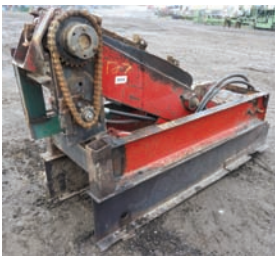
8059 $4,200.00 LOG TURNER chain type log turner, 36" chain, hyd drive, good working condition 260-633-4047
