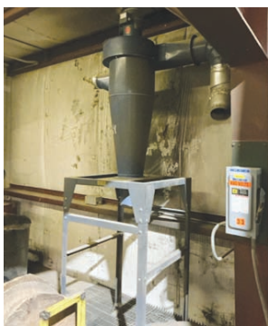
Blower, Pipe and Cyclone — Description — 18" blower and cyclone, 7" steel pipe, some 4" branches, approximately 100' total
