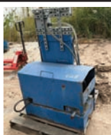
Hydraulic Pak — Description — 10 hp electric hydraulic Pak, solenoid valve and control panel
