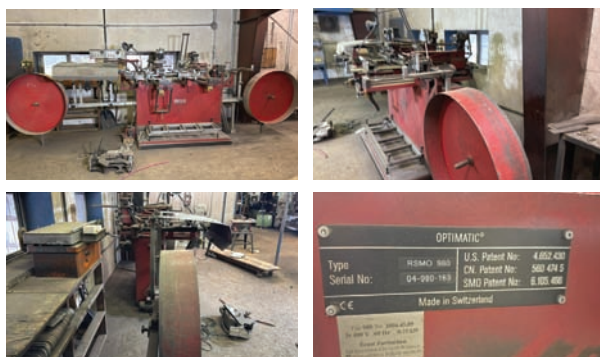
Simonds Automated Bench — Description — Simonds, SN 04-980-163, model RSMO-980, automated band leveler, level, tension, pull back, set tires
