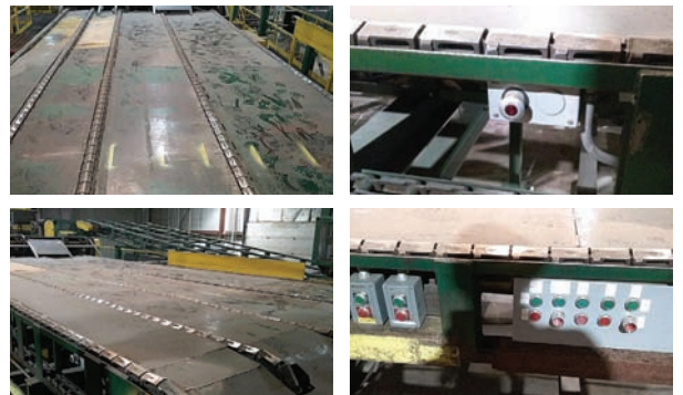
5 Strand Transfer Deck — Specifications & Features — Make: na. Drive Type: Electric. # of Strands: 5. Overall Dimensions: 11'x26'. Chain Type: H-130. — Seller Statement — Solid Steel decking, roof top chain
