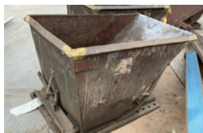
Self Dumping Hopper — Description — 36"x60"x32"
