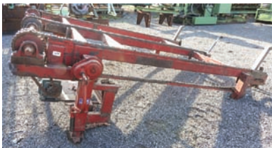
9286 TRANSFER DECK 3 strand transfer deck, 7' wide x 11' long, lineshaft ready, good working condition 260-633-4047
