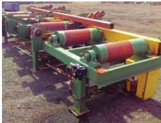
9281 ROLLCASE rollcase/ pop-up transfer, 30" wide x 13' long, 3 strand transfer, hyd and electric drive, has cant flippers, heavy duty and in excellent condition 260-633-4047
