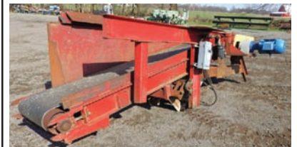
9291 DROP BELT CONVEYOR 24" wide x 11' long, electric drive, air cylinder for up-down movement, good working condition 260-633-4047
