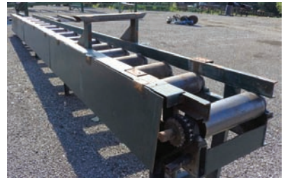
9313 ROLL CASE $3,750.00 18" wide x 25' long, heavy duty and in very good condition 260-633-4047
