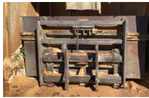
Dust Bucket — Description — 8' x 5' x 4", Welded on 22.5" x 20" quick attach frame, not a scraping style bucket, dumping hopper style.
