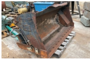
CAT High Dump Bucket — Description — 68" x 34" x 22" hyd dump. skid steer size quick attach
