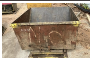
Self Dumping Hopper — Description — 54 1/2"x59"x32"
