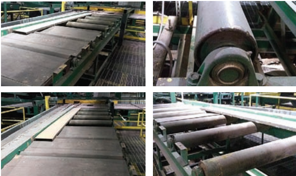
Rollcase — Specifications & Features — Make: na. Drive Type: Electric. Roll Spacing: 23". Roller Size: 6 1/2"x53 1/2". Overall Dimensions: 64"x228". Shaft Size: 2 1/2". — Seller Statement — Was not in use.
