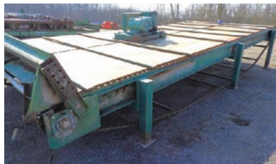
9290 SLAB DRAG WASTE CONVEYOR 10' 6" wide x 20' long, has steel slats to drag waste/ slabs, electric drive, good working condition 260-633-4047
