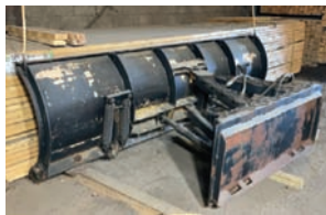
Snow Plow Blade — Description — 8' blade fits skid steer quick attach, power angle, spring loaded cutting edge.
