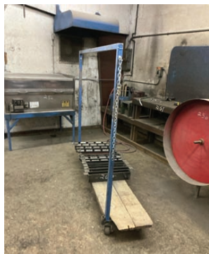
Chipper Knives and Cart — Description — Thirty Two 19 1/2" blades, Includes cart 83"x16"x57" tall
