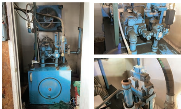
Hydraulic PAC — Description — 40 hp electric motor
