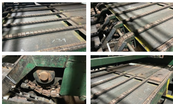
6 Strand Transfer Deck — Specifications & Features — Make: na. Drive Type: Electric. # of Strands: 6. Overall Dimensions: 9'x14'. Chain Type: MAC H78B Rooftop.
