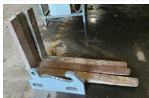
Lift Forks — Description — 3 pc. 5" x 48", fits 24" frame, 1 pc. quick attach bracket 17" c to c.
