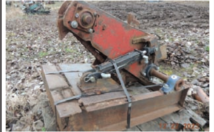
8052 $3,100.00 MEADOWS LOG TURNER Meadows 36" chain type Log Turner (Sawmill), hyd drive, working condition 260-633-4047
