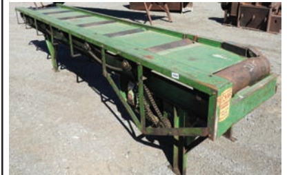
9284 LIVE ROLL CASE 24" wide x 15' long, electric drive, 6 1/2" dia rolls, good working condition 260-633-4047
