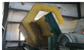
RENS Log Metal Detector — Description — Type 80-40, sn 091200, 14' feed thru trough, 40" coil, control box
