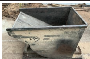
Self Dumping Hopper — Description — 34"x47"x25"
