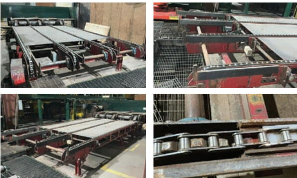
4 Strand Mellott Transfer Deck
