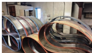
Double cut Bandsaw Blades — Description — 89 plate, VDP, 14 gauge, 2" space, 10 blades,
