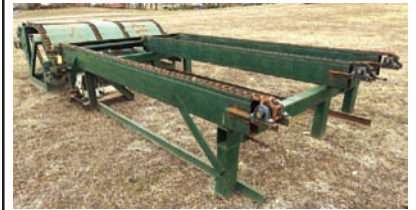
9280 UNSCRAMBLER/ TRANSFER DECK 3 strand transfer deck & unscrambler, deck is 8' wide x 13' long, both are gearbox drive, good condition and ready for production 260-633-4047
