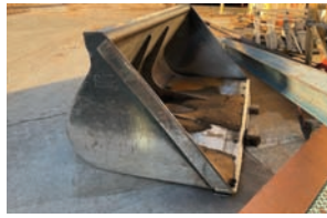
Cat Loader Bucket — Description — 8' x 40" x 40", 22.5" x 20" quick attach
