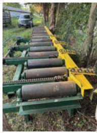
9303 ROLL CASE $7,500.00 24" wide x 20' long, 4 strand pop-up transfer, transfer goes both directions, hyd drive, heavy duty and in excellent condition, ready for production 260-633-4047
