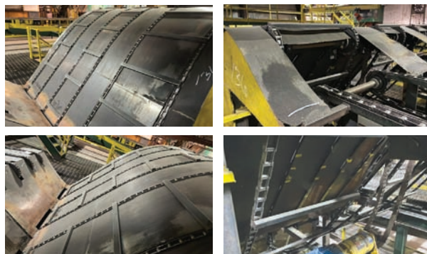
6 Strand Unscrambler — Description — 133"x110", 6 Strand, Electric drive
