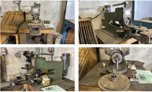
Williams & White Stretcher Roller — Description — SN 36330, model 36 EB, for circular saws
