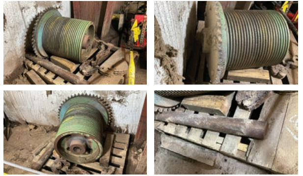
Cable Drum — Description — Carriage drive cable drum, new shaft, 20" drum 3 7/16" shaft,
