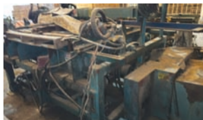
Pallet Stringer Notcher — Specifications & Features — Make: GBN. Model: Thena. Serial #: na. Drive Type: Manual. Heads: Double. Infeed: none. Length Capacity: 65". Indexable Teeth on Head: yes. — Seller Statement — No drive
