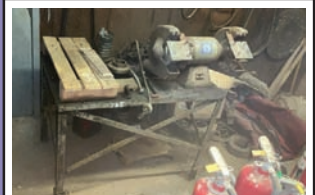
Grinder and Steel Table — Description — Table: 27 1/2"x40 1/2"x29", one hp. Electric motor on 8" grinder-buffer.
