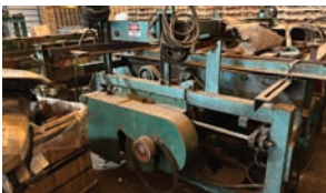
Pallet Stringer Notcher — Specifications & Features — Make: GBN. Model: Thena. Serial #: na. Drive Type: Manual. Heads: Double. Infeed: none. Length Capacity: 65". Indexable Teeth on Head: yes. — Seller Statement — No drive
