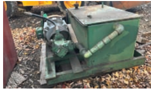
Hydraulic Pack — Description — 30hp electric motor, 55 gallon oil tank
