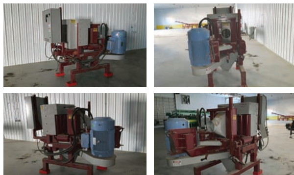
2017 Keystone Machinery Cant Sizer — Specifications & Features — Year: 2017. Make: Keystone Machinery. Model: VS-8-10 Vertical Sizer. Serial #: E-H-HY-40-V18-035. — Seller Statement — Looks like it has never been used. 16" vertical sizer head. 40 hp. electric motor.
