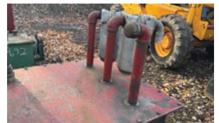
Hydraulic Oil Tank — Description — 165 gallon tank
