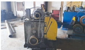
Roll Former — Description — Brand unknown, 3 8"x8'2" rolls 8'2" capacity, electric drive, 15 hp 3 phase electric motor, electrical controls need some work
