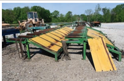
9205 $4,000.00 ROLL CASE Roll case/ transfer deck, rolls are 30" wide x 38' long total length, transfer is 52" wide and 38' long, lighter duty and in good working condition 260-633-4047
