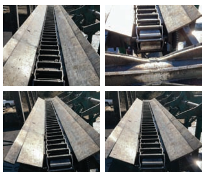
Infeed Log Trough — Specifications & Features — Make: Morbark. Drive Type: Hydraulic. Size: 38" x 20'. Overall Width: 42". Pan Width: 14". Log Kickers: no. Chain Type: Ladderback. — Seller Statement — Shop built, good trough, Supports to ground
