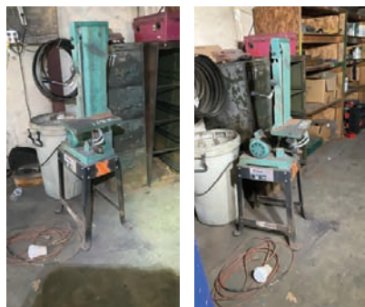
Grizzly Combination Sander — Description — 6" x 22" flat belt vertical or horizontal, disc is missing
