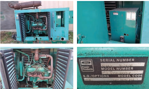
Onan Genset — Specifications & Features — Engine Year: unknown. Engine Model: LS6-8751-6003-6. Engine Make: Ford. Engine Number: 12483 H-29-RL. Fuel: LP. Meter Reads: 825 hours. Generator Make: Onan. Generator Model: 100ENBA. Generator SN: H930516504. Capacity (KW): 1 phase 67, 3 phase 100 KW. — Seller Statement — Runs and Operates
