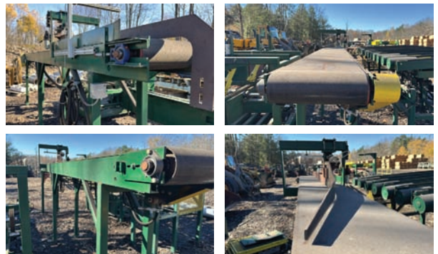
Belt Conveyor — Specifications & Features — Drive Type: Hydraulic. Length: 19'. Overall Height: 88". Overall Width: 26". Belt Width: 20". — Seller Statement — Laser, board diverter
