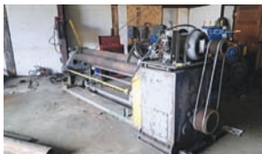
Roll Former — Description — Brand unknown, 3 8"x8'2" rolls 8'2" capacity, electric drive, 15 hp 3 phase electric motor, electrical controls need some work
