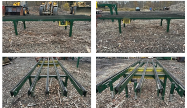
Transfer Deck — Specifications & Features — Make: na. Drive Type: Hydraulic. # of Strands: 5. Overall Dimensions: 4'x16'x35"high. Chain Type: link. — Seller Statement — With air stop n go
