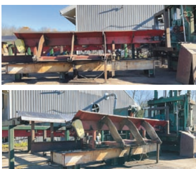
Outfeed Log Trough with Kickers — Specifications & Features — Make: Morbark. Drive Type: Hydraulic. Size: 52" x 20'. Overall Width: 7'. Pan Width: 14". Log Kickers: yes. Chain Type: Ladderback. — Seller Statement — 3 kicker arms, kicker joints show some wear, support to ground
