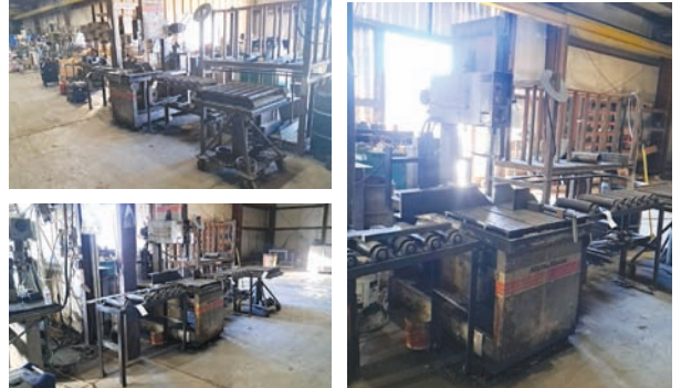
Metalmizer Bansaw — Description — Model#MS2018, SN# MS0289022, 1" band, electric drive General Electric 2 hp 3 phase electric motor, 3 roll cases included
