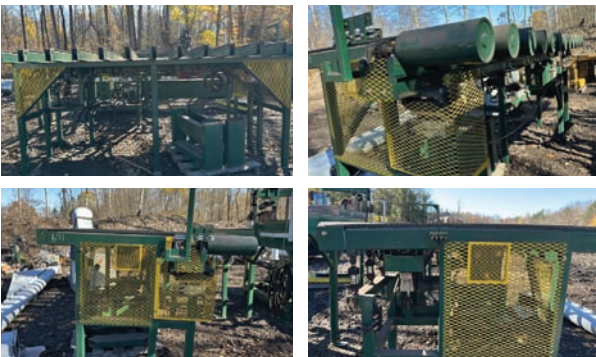
Transfer Deck — Specifications & Features — Make: unknown. Drive Type: Hydraulic. # of Strands: 13. Overall Dimensions: 147"x77"x67"high. Chain Type: link. — Seller State- ment — One side has live rollcase with pop up
