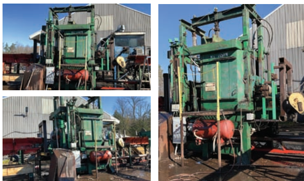
Nicholson Ring Debarker — Specifications & Features — Year: na. Make: Nickolson. Model: A1-27. Serial #: na. Head Driven by Electric: yes. Power Pack: yes. # of Arms: 6. Roller Tensioner Arms: Hydraulic. Size: 27". Cab: no. Controls: Joystick. Log Capacity: 30'. Feed Rolls Powered by: Hydraulic. — Seller Statement — Controls in Cab, cab not included, good working condition.
