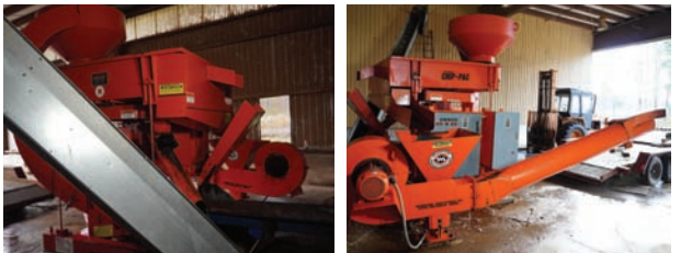
Morbark ChipPak — Specifications & Features — Make: Morbark. Model: 48. Powered by: 75 hp. electric. Size: 48". Screen Size: 5'. — Seller Statement — Includes cyclone, 75 hp. Electric motor, 3 knife, shows very little use. Shaker is on rods.
