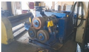
Buffalo Forge Roll Former — Description — 7" rolls, 20 hp electric motor
