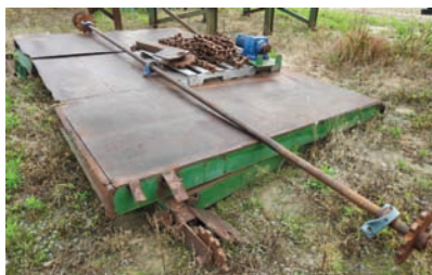
9223 $8,500.00 SLAB DRAG DECK slab drag conveyor, 15' x 14', electric gearbox drive, 81X chain with steel cleats bolted on, good condition 260-633-4047
