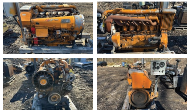
Deutz Power Unit — Specifications & Features — Year: 1999. Make: Deutz. Model: BF6L913C. Serial #: DIN/ISO 3046 IF N. Engine Cylinder: 6.0. Fuel: Diesel. Meter Reads: na. Horsepower: 177. Clutch: no. — Seller Statement — Running condition unknown
