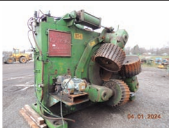
6045 $57,500.00 RING DEBARKER 30" dia Cambio ring debarker, 6 arms, steel infeed press wheels, all electric, all electrical and controls included, recently in production and in good working condition, infeed/ outfeed also available, call for price 260-633-4047
