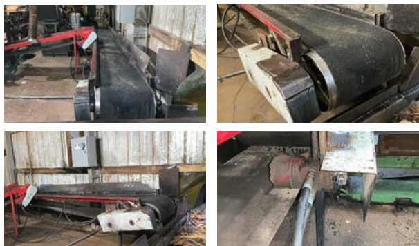
Belt Conveyor — Specifications & Features — Drive Type: Hydraulic. Length: 32'. Overall Height: slight incline to 39". Overall Width: 24". Belt Width: 18". — Seller Statement — 80" slider chute on end
