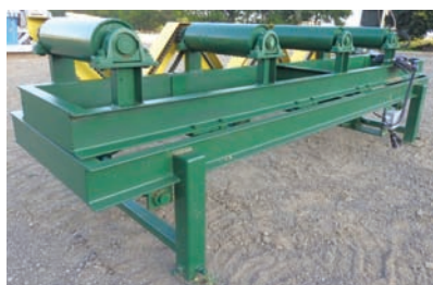
9217 $4,500.00 ROLL CASE rollcase, pop-up rollers, perfect for putting in a transfer deck, 16" wide x 7' long, foot pedal control, hyd drive, BRAND NEW! 260-633-4047
