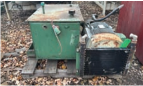
Hydraulic Pack — Description — 30hp electric motor, 55 gallon oil tank
