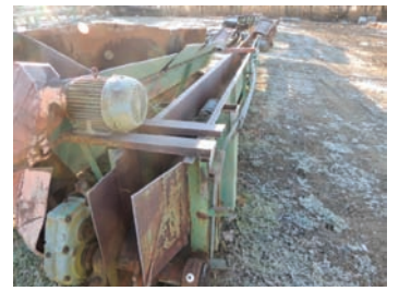
9142 WASTE CONVEYOR $8,500.00 10"x60' waste conveyor H78 chain with paddles, electric drive, includes new chain 260-633-4047
