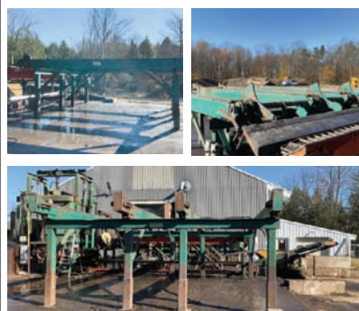
Winston Machinery Log Deck — Specifications & Features — Make: Winston Machinery. Drive Type: Electric. Up & Down Cylinder: Hydraulic. # of Strands: 4. Stop'n'Load: yes. Size: 17' x 21'6" x 92". — Seller Statement — Heavy duty deck, Support to ground.
