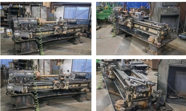
1941 Monarch Lathe — Description — Sn#J-240-N, 18.5" swing 78" between centers, electric drive
