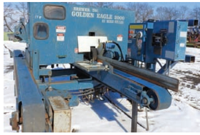
3093 $15,000.00 RESAW Brewer Golden Eagle single head resaw, electric drive, 36" dia wheels, return belt, includes numerous extra blades, this machine is in excellent condition and ready for production 260-633-4047
