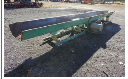
9240 VIBRATING CONVEYOR $7,500.00 Webster vibrating conveyor, 18" wide pan x 20' long, electric drive, good working condition 260-633-4047
