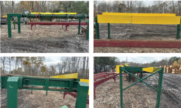
Transfer Deck — Specifications & Features — Make: na. Drive Type: Electric. # of Strands: 5. Overall Dimensions: 8'x18.5'x80"high. Chain Type: H 78 B rooftop.
