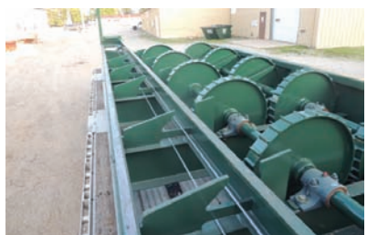
6048 $87,500.00 DEBARKER Precision rosser head debarker, Model P636, Serial # D563, 36" capacity, electric drive on head, self-contained hyd unit for carriage etc., upgraded to chain drive for carriage, price is Showcase Rebuilt and comes with warranty. CURRENTLY IN THE SHOP SO CALL WITH YOUR SPECS TO HAVE IT CUSTOMIZED! pics similar to actual machine 260-633-4047
