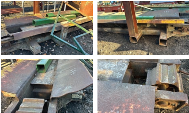
Conveyor Section — Description — 11', overall width is 44", with a 14" pan, no drive
