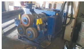
Buffalo Forge Roll Former — Description — 7" rolls, 20 hp electric motor
