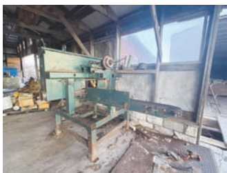
3627 $4500 SINGLE HEAD KENT RESAW 6" wide opening, cable clutch, and roller guides. Lineshaft ready and in good working condition. MAKE AN OFFER TODAY. 574-536-1646
