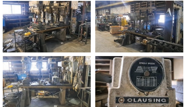
Clausing Drill Press — Description — 4 head drill press, model#2233, Sn#512114, electric drive, no power
