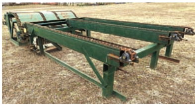
9280 $10,500.00 UNSCRAMBLER/ TRANSFER DECK 3 strand transfer deck & unscrambler, deck is 8' wide x 13' long, both are gearbox drive, good condition and ready for production 260-633-4047
