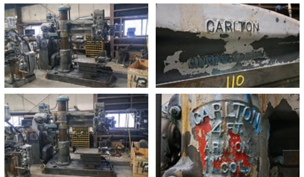
Carlton Drill Press — Description — 11"x4' capacity, electric drive
