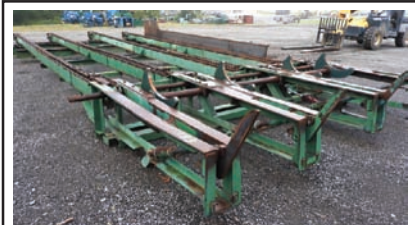
9321 $10,500.00 LOG DECK Edmiston log deck, 4 strands 12' wide x 34' long H-78 chain, stop-load, good working condition 260-633-4047
