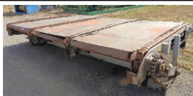
9316 $3,750.00 TRANSFER DECK 4 strand transfer deck, approx 9' wide x 8' long, H-78 rooftop chain, electric drive, good condition 260-633-4047
