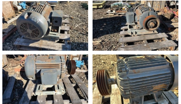
Electric Motor — Specifications & Features — Make: Baldoe Reliancer. Horsepower: 100. Phase: 3 Phase. Frame Size: 405T. RPM: 1775.
