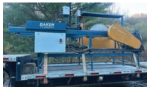
Baker Scragg Mill — Description — Single blade cant splitter. Log holding carriage, — Contact — Specialist: Myron Nissley, 574-536-2481.
