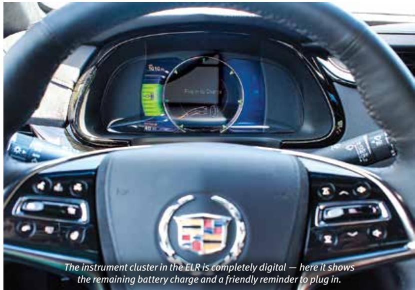
The instrument cluster in the ELR is completely digital — here it shows the remaining battery charge and a friendly reminder to plug in.
