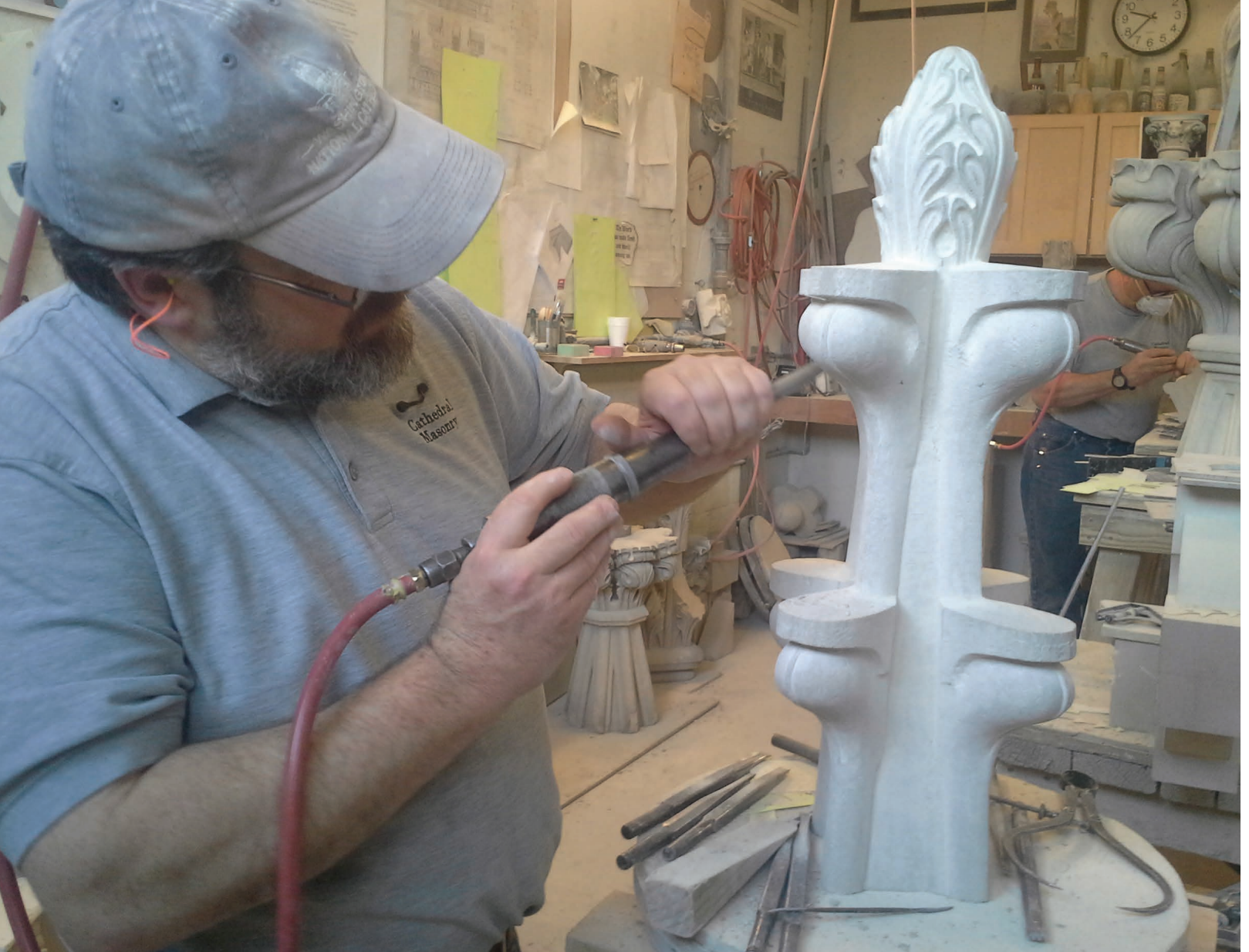
Sean Callahan, a cathedral stone carver, finishes one of the rough cuts done by robotic carving. It takes about eight weeks to go from rough to ready. Photo courtesy Wiss, Janney, Elstner Associates
