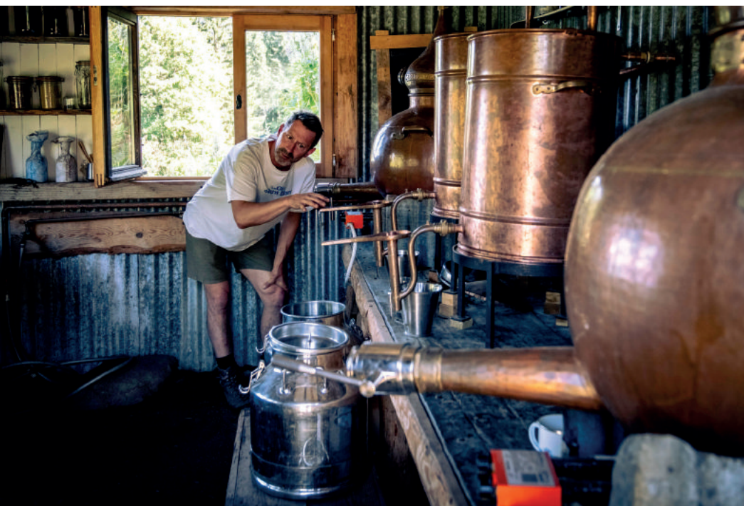
Two 100-litre gas-fired copper pot run on bottled gas rather than electricity – essential given frequent power cuts (Photo: Distilleries Saint Gervais)
