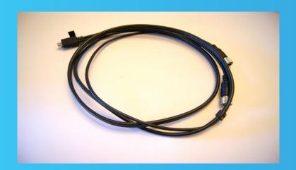
Connect the end of the Micro USB cable to the camera. Next, connect your 6 pin M8 male receptacle end to the OBD to M8 female receptacle as show in the image.
