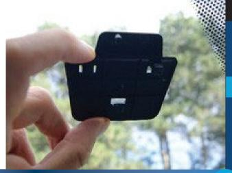
Attach the camera to the mounting plate by matching the positions of the three mounting holes on the back of the camera with the hook on the rear plate. Slide the camera to the left to lock it in place.
