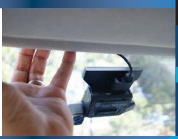
Route the cable along your windshield frame, ensure the cable is tucked alongside existing wires of the pilar and behind pilar air bag.
