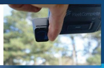
Using the Allen key, loosen the camera lens screws so you can adjust your lens positioning. Fasten your screws only once you have completed the Vision camera alignment steps from page 7.
