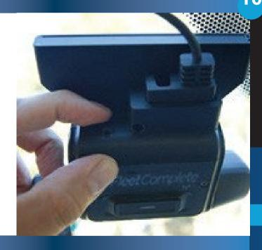
Screw in the peripheral cover with the Allen key provided to secure the camera and prevent damage.
